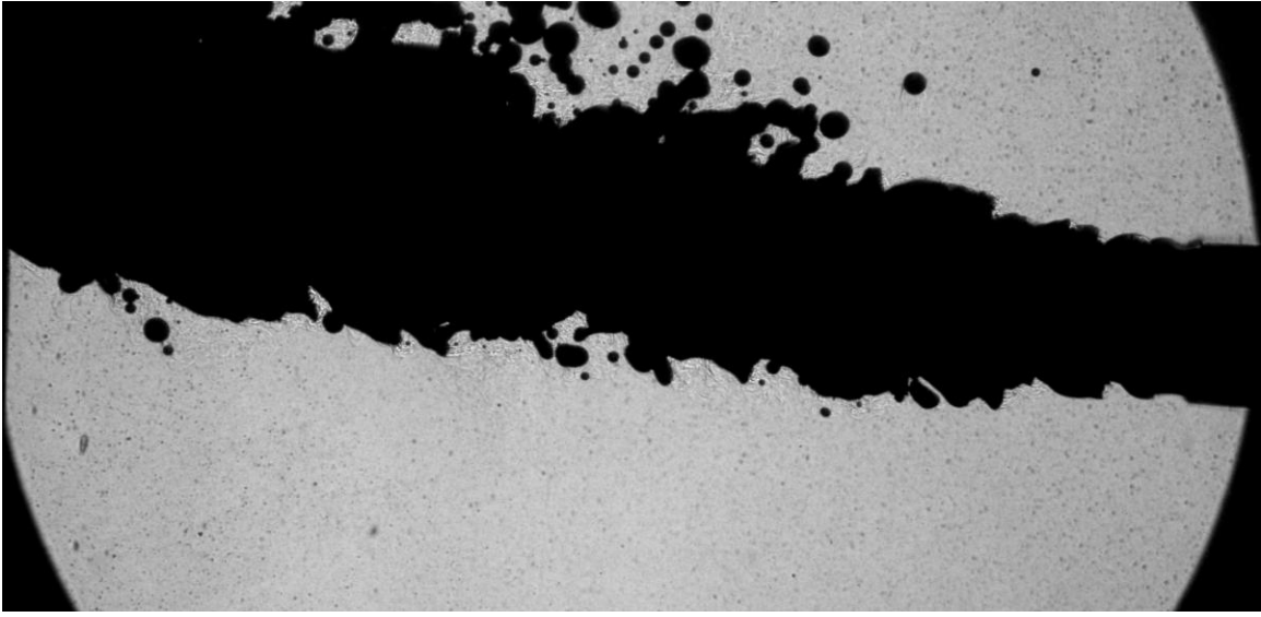
Figure 5. Schlieren/shadow photographs of 5 cs, 0.92 \text{ g/cm}^3 n=1.49 oil discharging horizontally into water tank.
