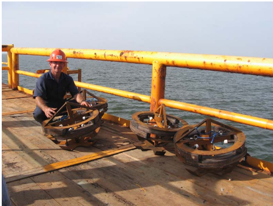
Photo#2: Scorpion™ Pile Severing Device with installed Engineered Charges (LSC's)
