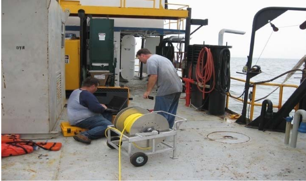
Photo #6: MMS personnel Mr. T. J. Broussard and Mr. Tre Glenn Setting up Mesotech Sector Scanning Sonar on Deck of the Seabream.
