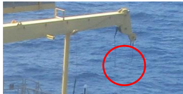
Figure 2 – Crane missing main block and auxiliary ball
