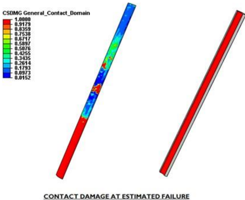
FIGURE 59: LARGE SCALE CONTACT DAMAGE AT ESTIMATED FAILURE UNDER COMBINED LOADING
