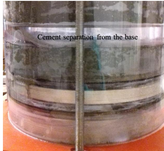
Figure 4.17: Cement separation during the 40-psi pressure test.
