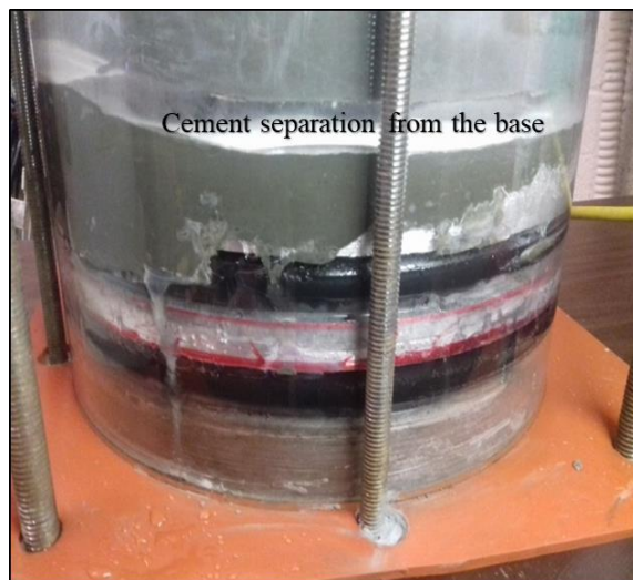
Figure 4.25: Cement separation during the 20-psi pressure test.
