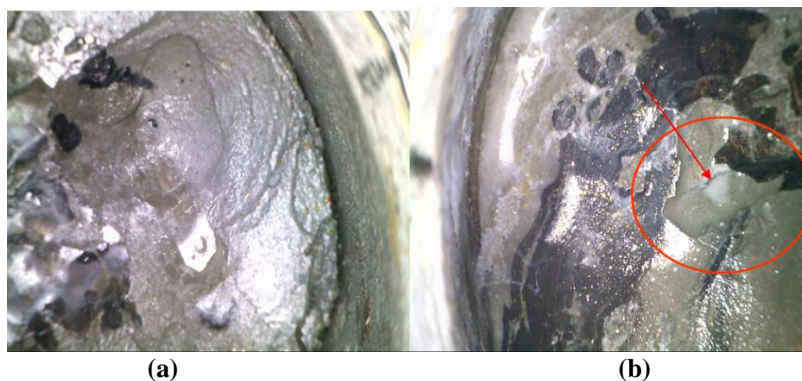
Figure 2.21: Nanomaterial cement sample before test without leaks (a) and during the test showing position 1 within the cement
