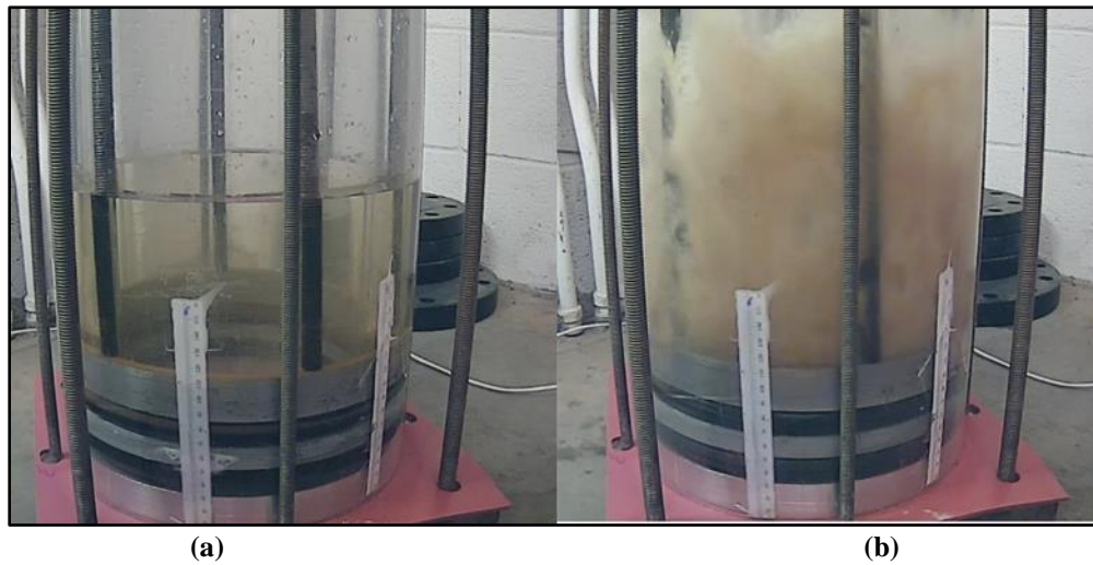
Figure 4.5: NBR before (a) and after (b) failure during pressure cycling
