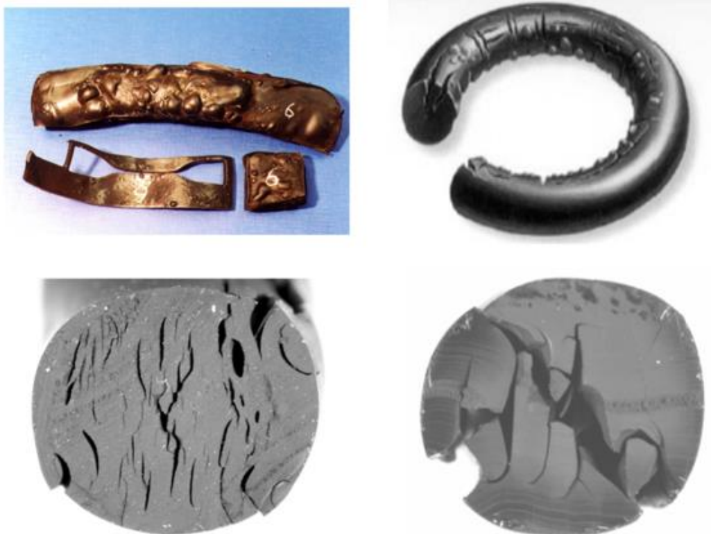
Figure 4. Some examples of elastomer failure caused by RGD (top row) and overload pressure (bottom row).
