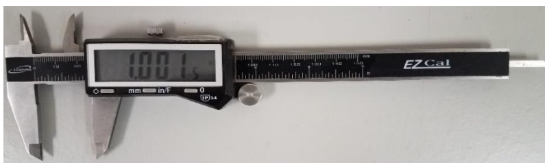
Figure 3.12: Digital Vernier Caliper.
