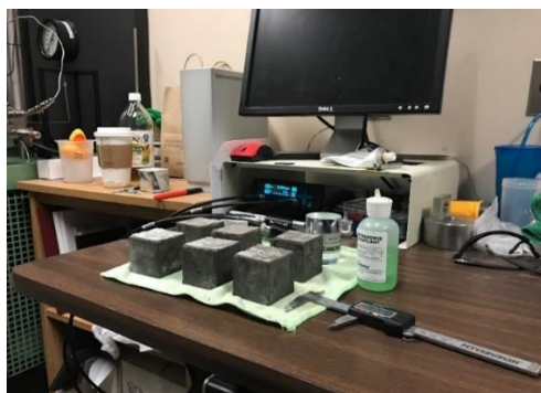
Figure 2.45: Dimensions of cement samples (Class H and Class G) measured.
