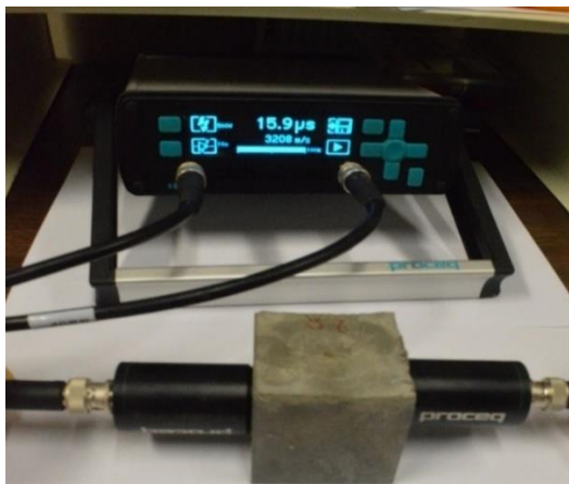
Figure 2.46: Ultrasonic cement test being carried out.
