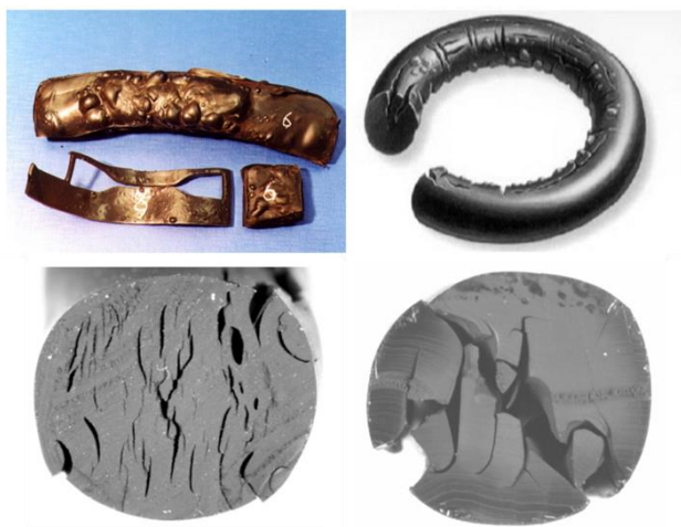
Figure 3.1: Some examples of elastomer failure caused by RGD (top row) and overload pressure (bottom row).
