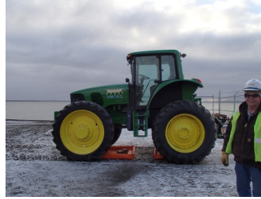
Tractor for Launching Vessels
