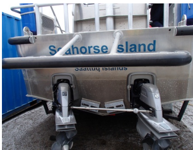
All Vessels - Twin Outboard Motors
