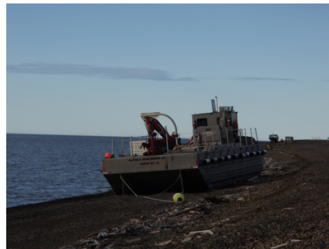
Mini-barge – 650 bbl capacity
