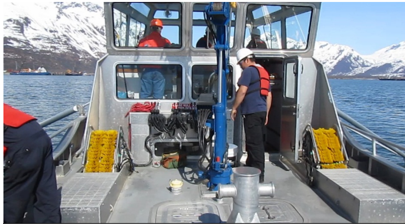
LORS-2 Brush Skimmer System on 47' Workboat Arctic Skimmer 1
