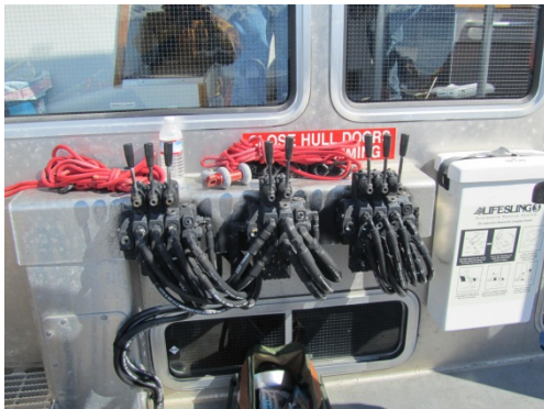
LORS-2 Skimmer System Controls
