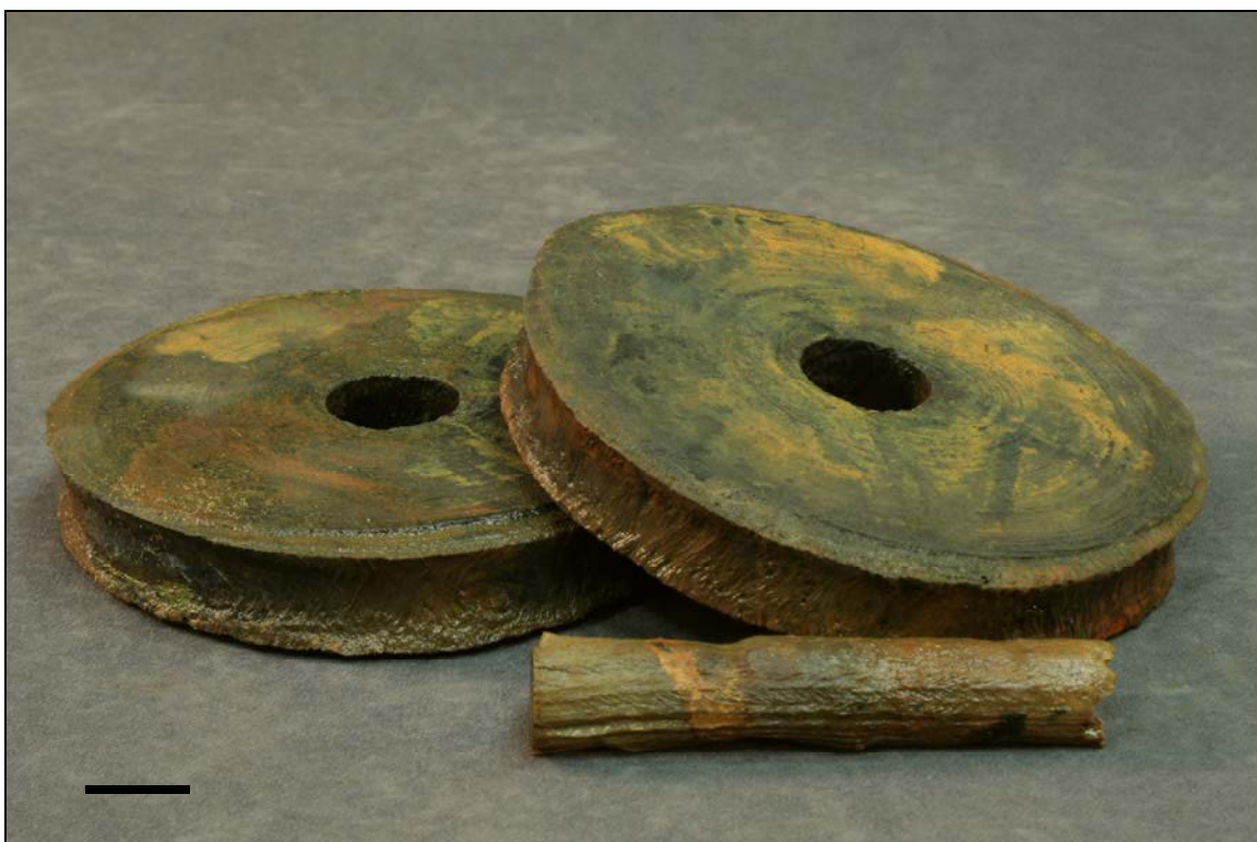
Figure 5.34. Double sheave and pin (artifact no. 140-1) recovered in double-block configuration (bar equals 2 cm; photograph by R. Sasaki).
