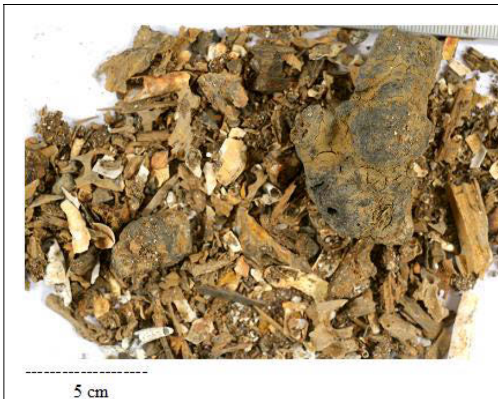
Figure 2.6. Total coarse fraction of core 1. The large object with a hole in its top is a concretion or a fluid expulsion feature.
