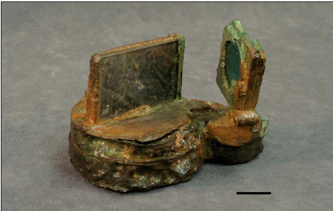
Figure 5.71. Octant index mirror assembly (artifact no. 133) (bar equals 2 cm; photograph by R. Sasaki).
