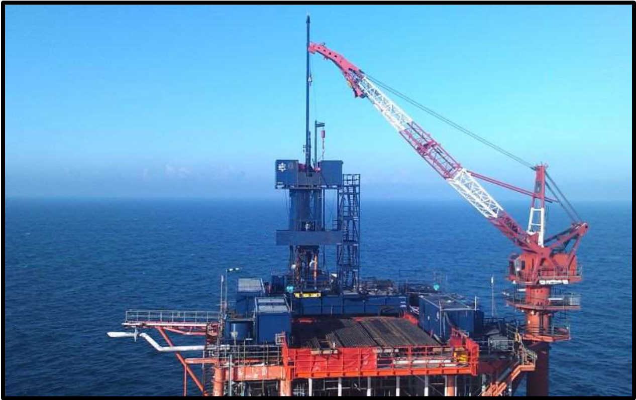
Figure 6-8. Hydraulic Workover Unit
