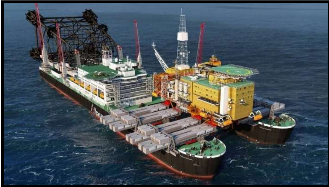
Figure 6-35. Allseas Pioneering Spirit Lifting System Topsides/Jacket (Drawing courtesy of Allseas)
