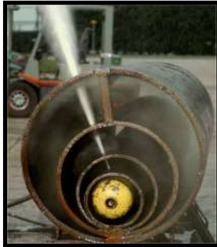
Figure 6-20. Water abrasive Cutting c/w internal manipulators
