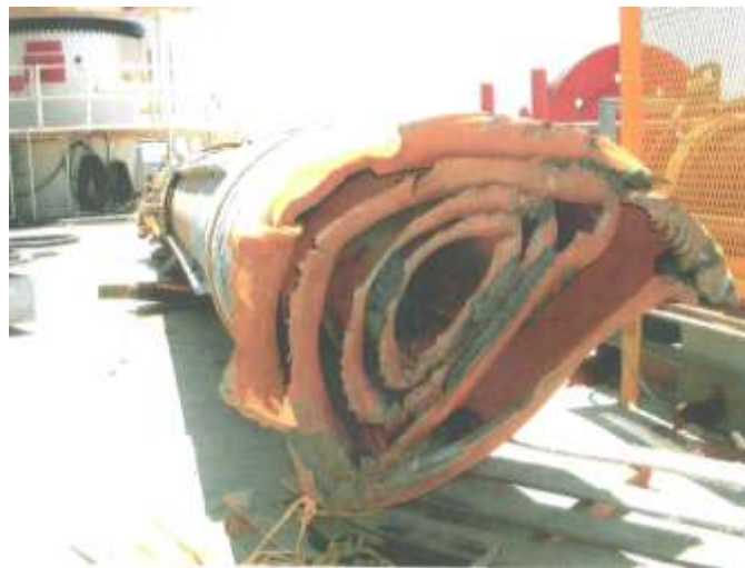
Figure 6-24. Multi-string Conductor Sheared below the Mudline (Photo courtesy of Prime Marine Services, Inc.)
