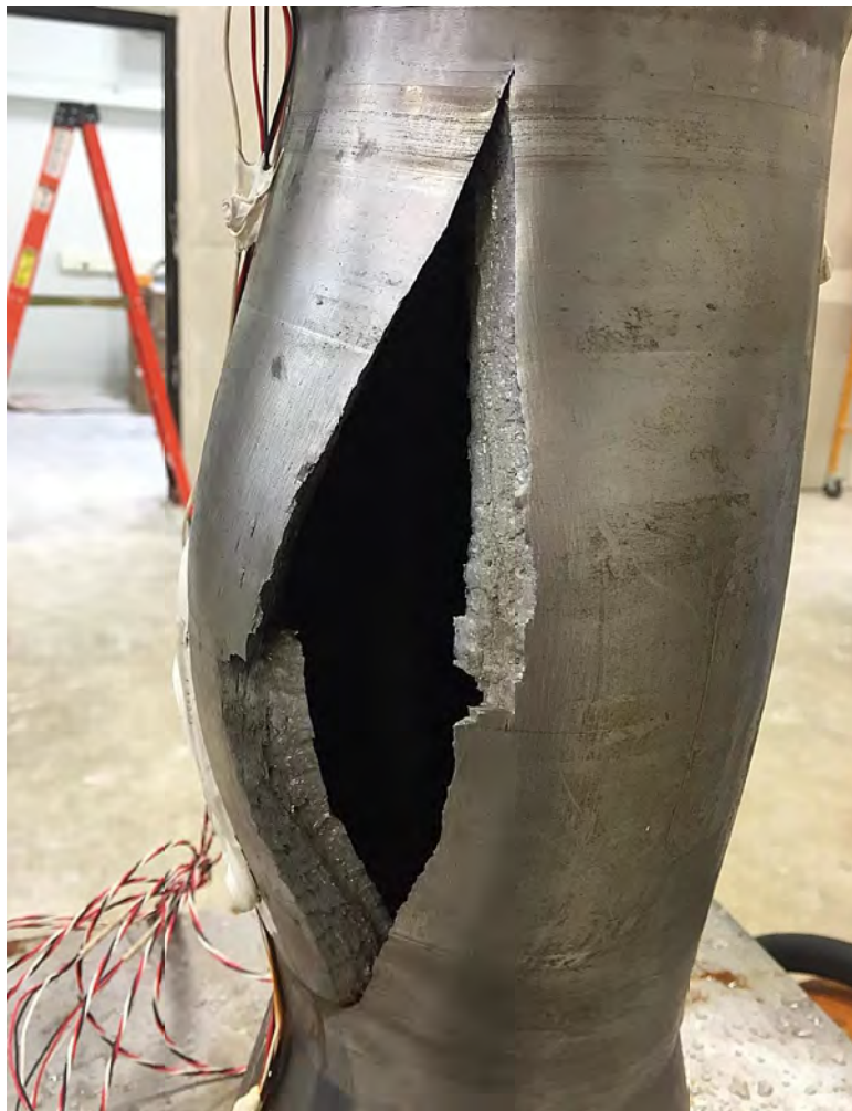
Figure 6.5 Rupture Failure in Small Test Body
