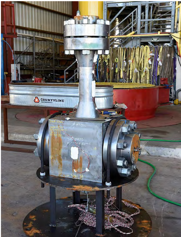
Figure 6.2 Assembled Test Body Ready for Testing
