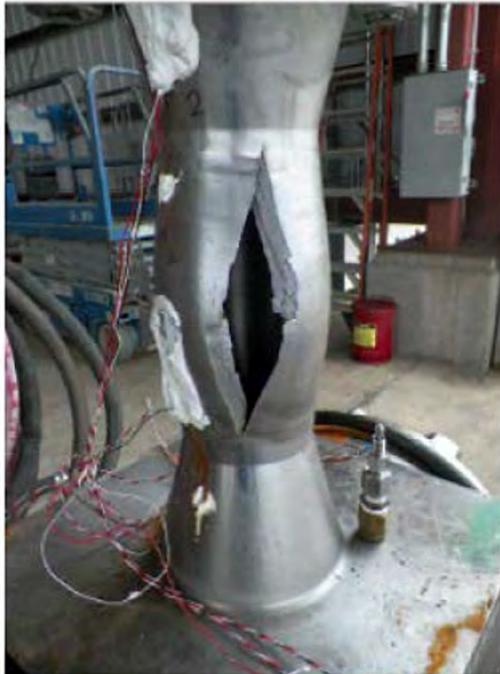
Figure IV-8. Large Valve Body Neck After Burst Test.
