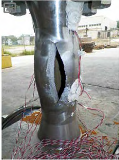
Figure IV-7. Small Vain Body Section After Burst Test.
