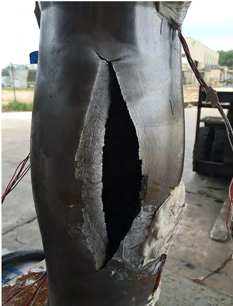
Figure 6.4 Rupture Failure in Large Test Body
