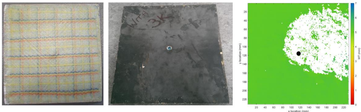
Figure 6. DRS inspection of a blow-off test plate sample. Green shows the steel WT where the composite remains bonded, white shows where the DRS signals are lost due to delamination.
