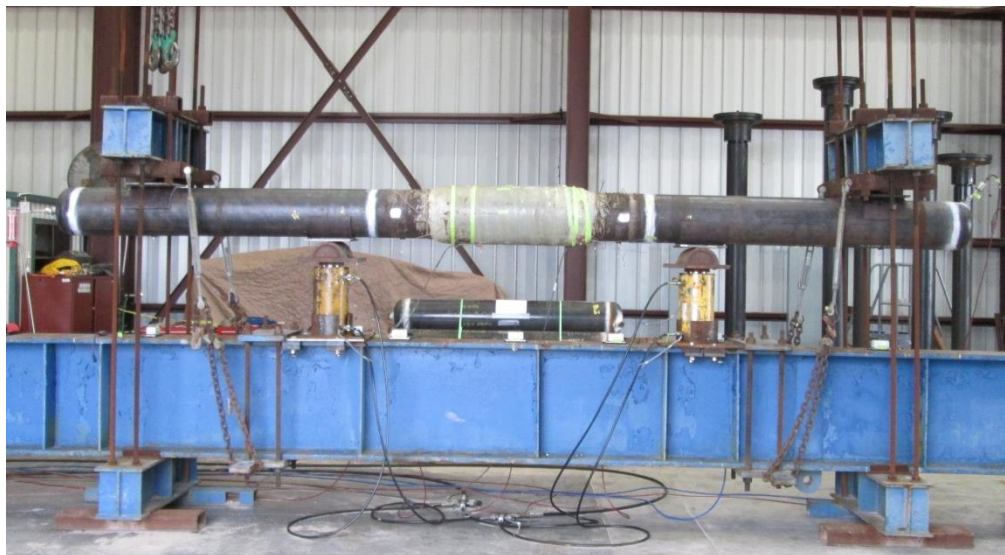
Figure 5-22: Manufacturer A's bending sample (OFF-A-BE-J2-4) installed in four-point load frame pre-test
