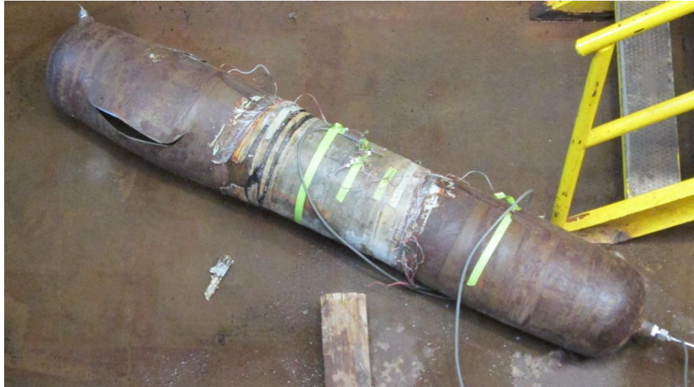
Figure 5-2: Manufacturer B's burst sample post-test – failure outside the composite
