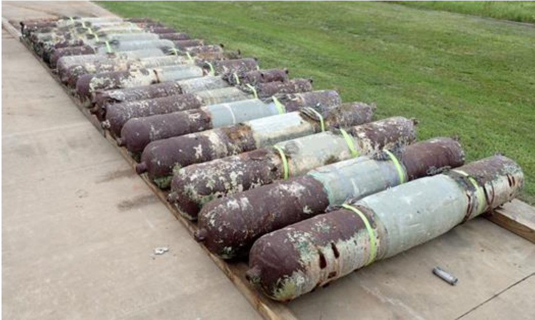
Figure 4-5: Photograph of samples after cleaning with pressurized water in preparation for the 90 day UV exposure.
