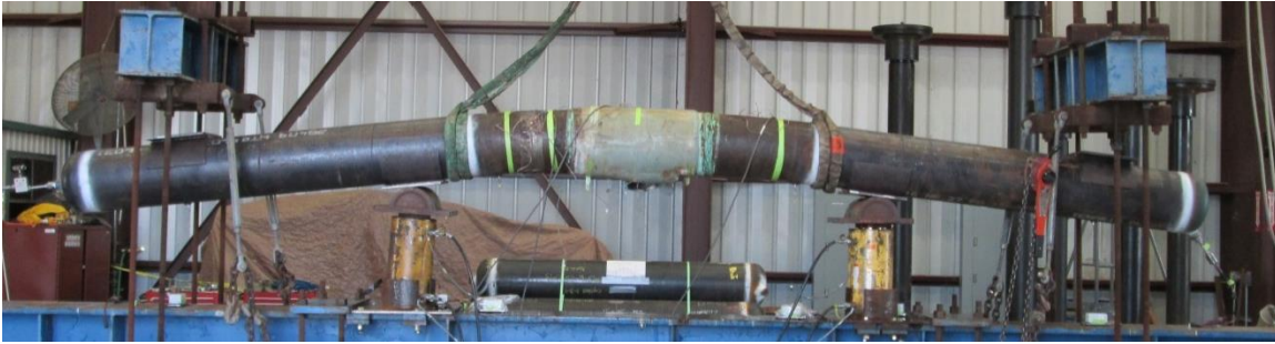
Figure 5-37: Permanent shape of Manufacturer C's bending sample (OFF-C-BE-J1-4) post-test (no bending load applied to sample at time of photograph)
