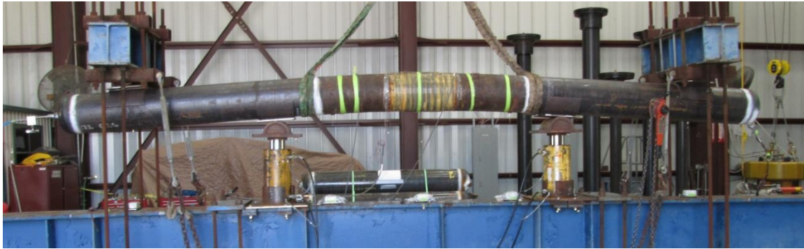
Figure 5-32: Permanent shape of Manufacturer B’s bending sample (OFF-B-BE-J2-4) post-test (no bending load applied to sample at time of photograph)
