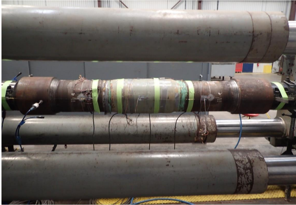
Figure 5-12: Manufacturer C's tension sample (OFF-C-T-J3-3) installed in 1-million pound load frame
