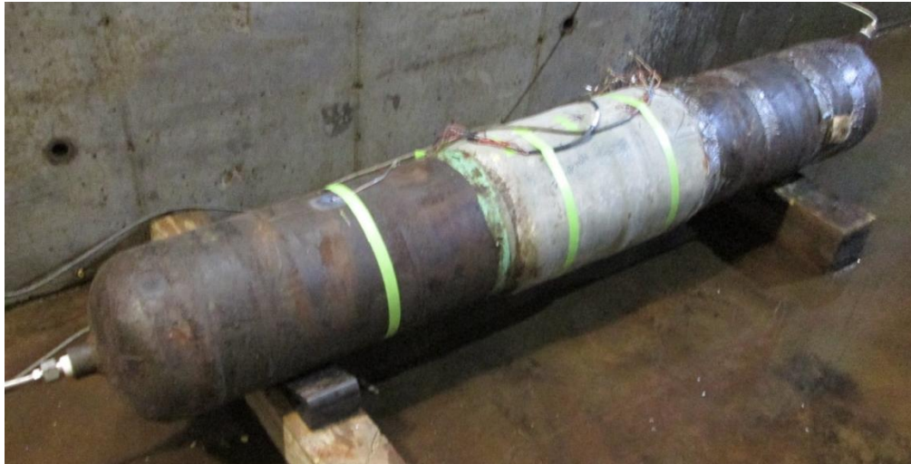
Figure 5-1: Manufacturer C's burst sample (OFF-C-B-J1-1) installed in test pit prior to burst test
