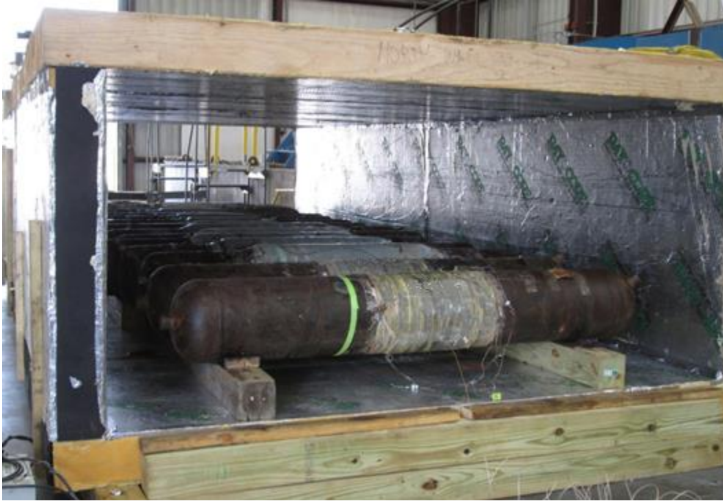
Figure 4-6: Photograph of insulated wooden box.
