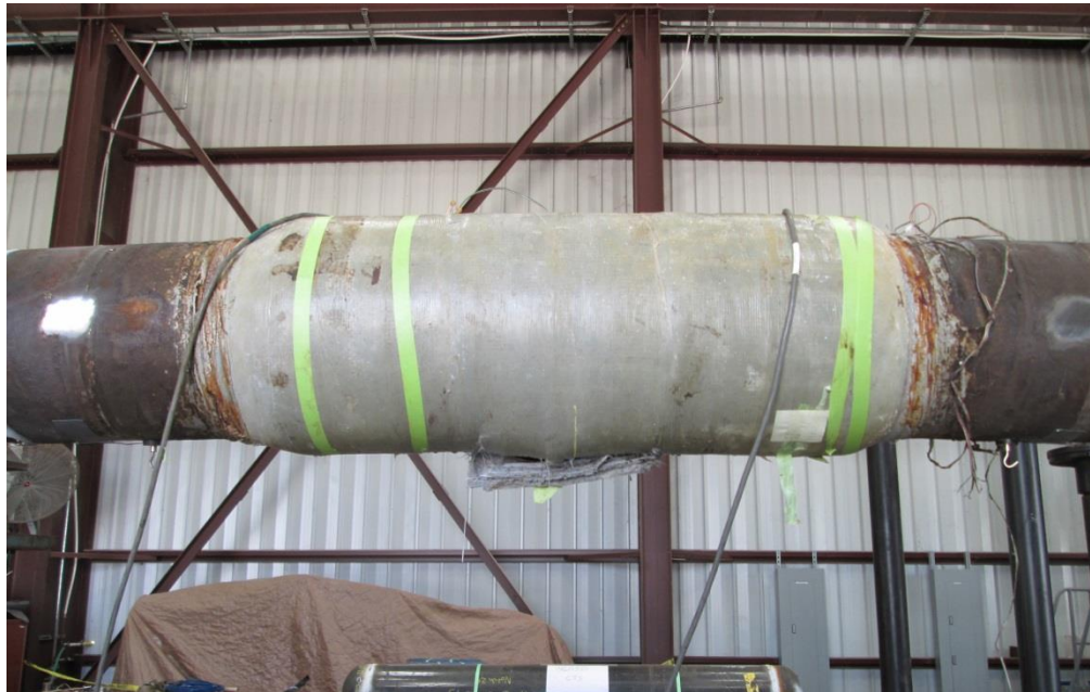
Figure 5-27: Failure at the corrosion defect in Manufacturer A’s bending sample (OFF-A-BE-J1-4)
