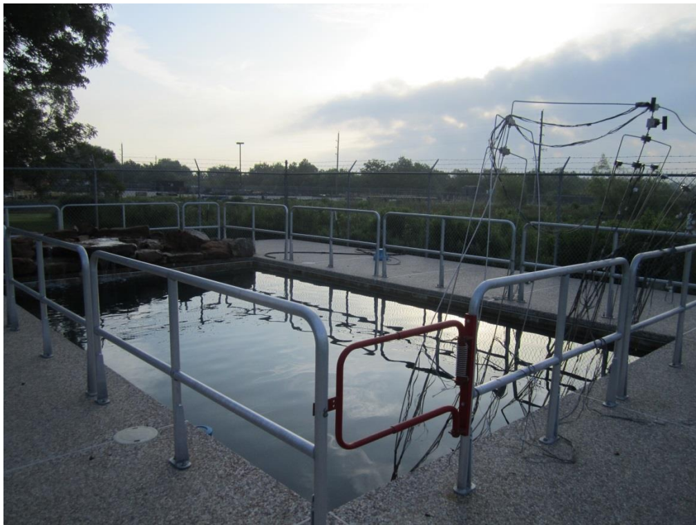
Figure 4-2: Simulated saltwater exposure tank at SES – Waller Test Facility
