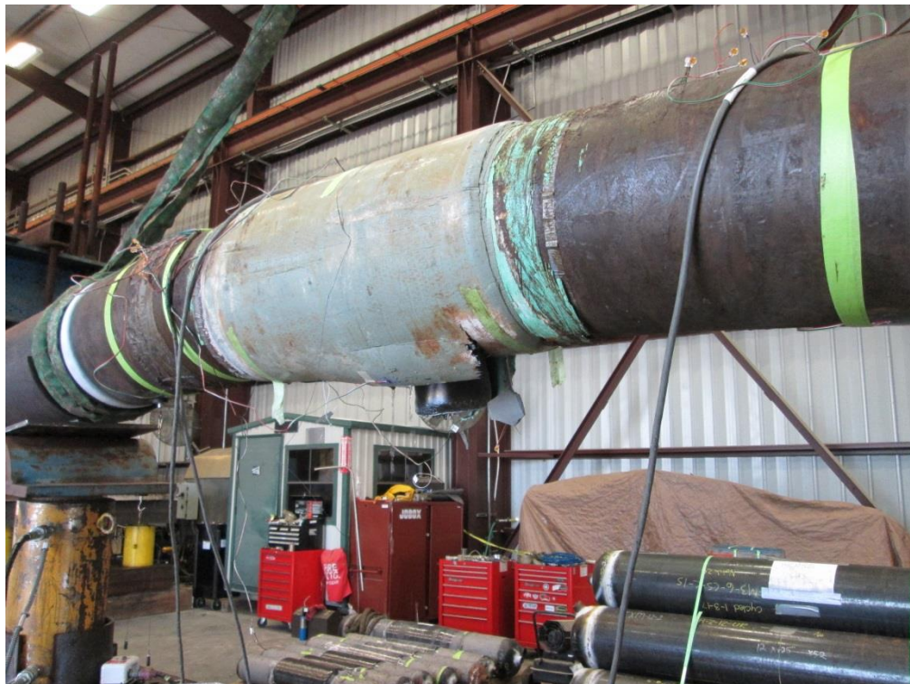
Figure 5-38: Failure at the corrosion defect in Manufacturer C's bending sample (OFF-C-BE-J1-4)
