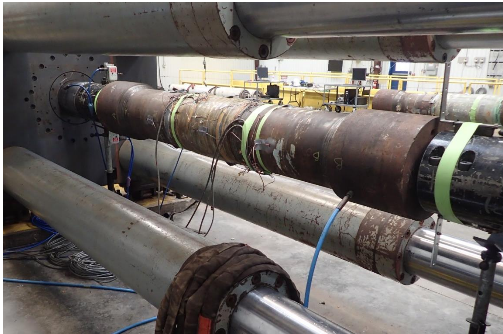
Figure 5-11: Manufacturer B's tension sample (OFF-B-T-J2-3) installed in 1-million pound load frame
