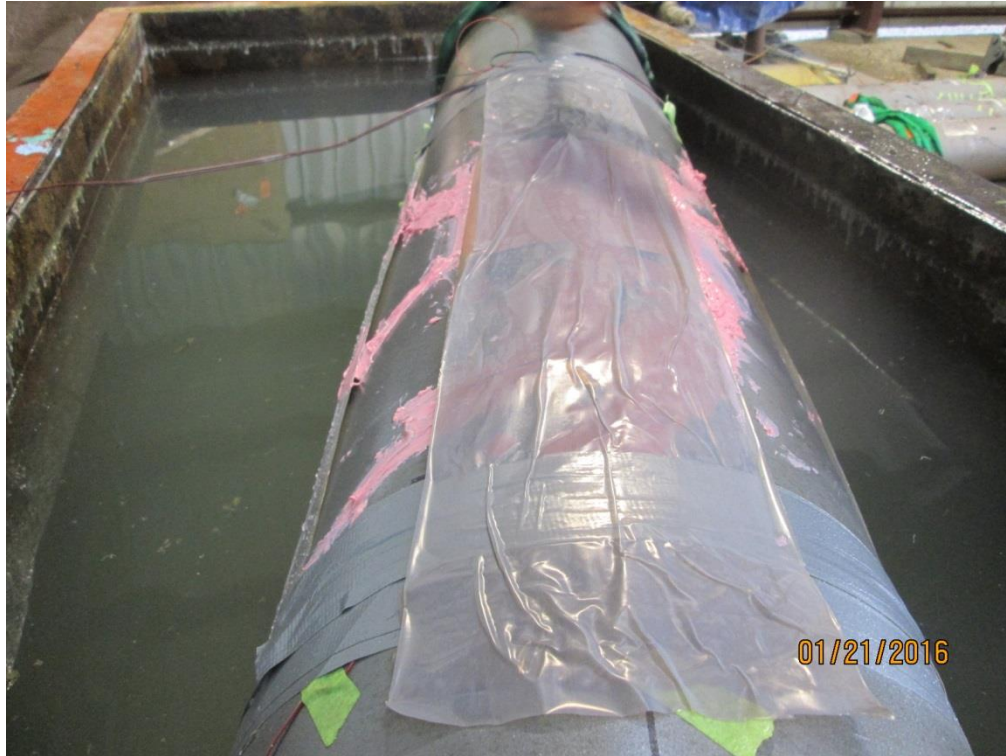
Figure 3-7: Example of artificial delaminations on Manufacturer B's sample (1 of 2)
