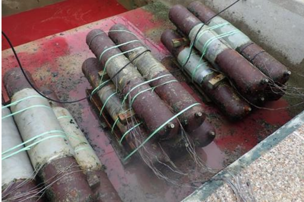
Figure 4-4: Photograph of samples after completion of 10,000 hour hold.
