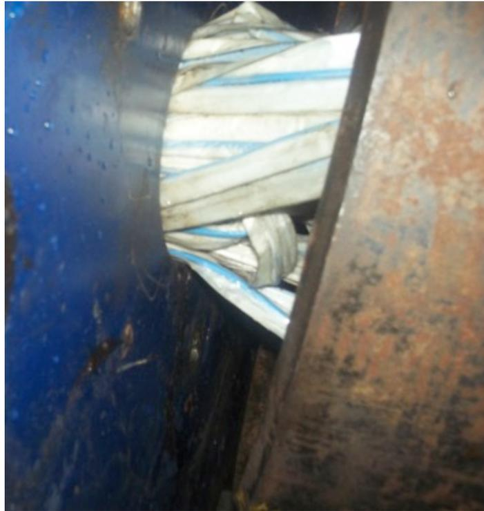
**Figure 35 Obstruction cap showing the copper coated wing wire slipping through the opening**
