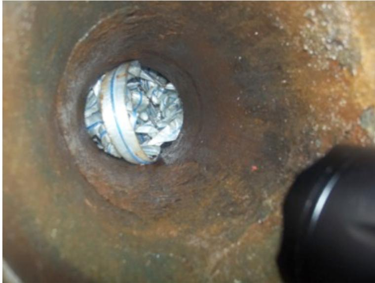
**Figure 29** Image from view port showing TWM still remains in place at 5.3 bbl/min.
