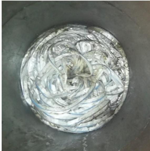
Figure 34 Image from inside the flow chamber showing that most of the TWM material was extruded by the flow under 81 psi of back pressure.
