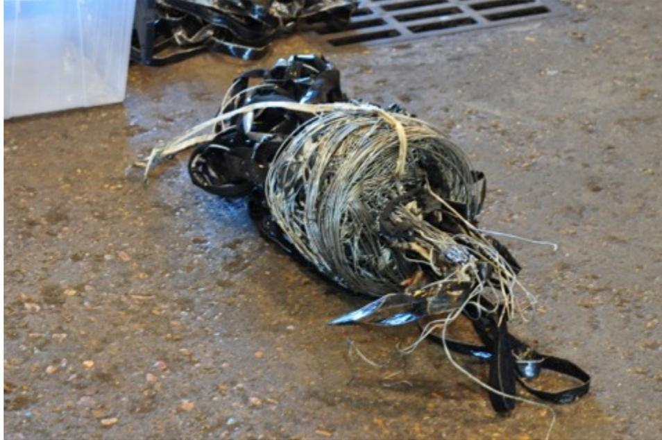
**Figure 45 TWM from test 7 material remaining inside the flow chamber after tested till 11,000 psi**
