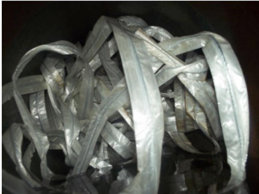
**Figure 32 Strengthening material still loos in the flow chamber**
