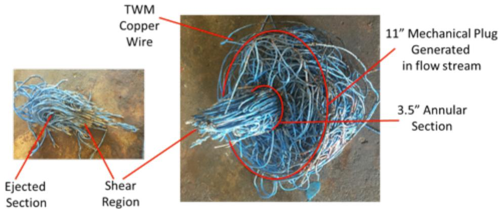
Figure 23 Tangled wire mass made from copper wire using a 3.5" open annular obstruction. The TWM sheared at a differential pressure of ~1,500 psi (2,250 observed at the pump).
