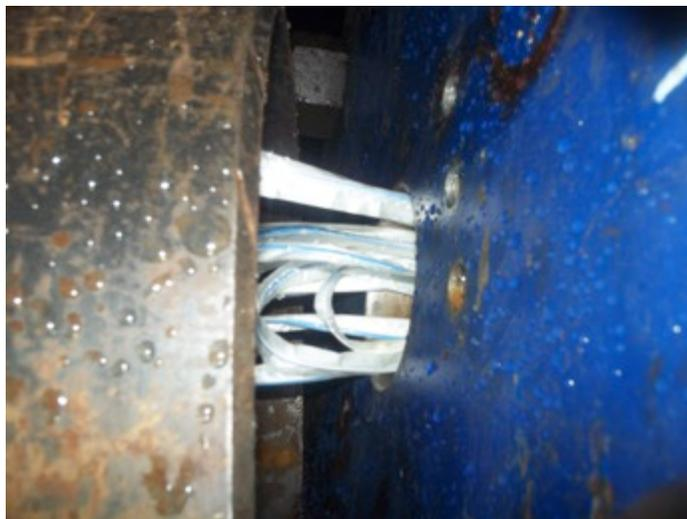
**Figure 31 Scaffolding material at the obstruction flange. Thus showing that the TWM has travelled to the obstruction and started the anchoring process.**
