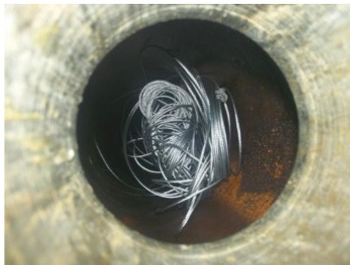
**Figure 46 AC 1/8 inside flow chamber viewed from the obstruction flange aperture**
