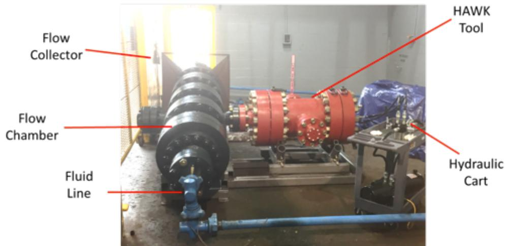
Figure 14 Test setup showing HAWK tool connected to flow chamber
