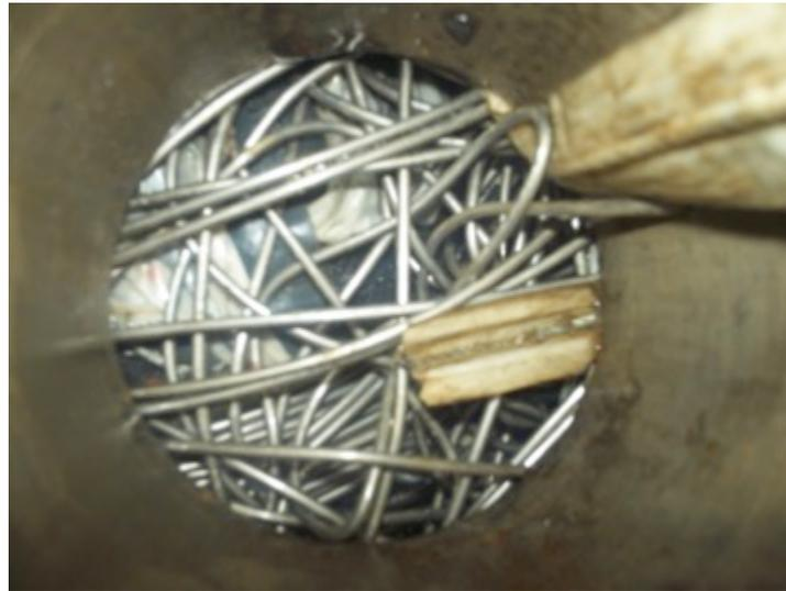
**Figure 40 Figure showing the TWM at the obstruction flange from the 3.5” port.**
