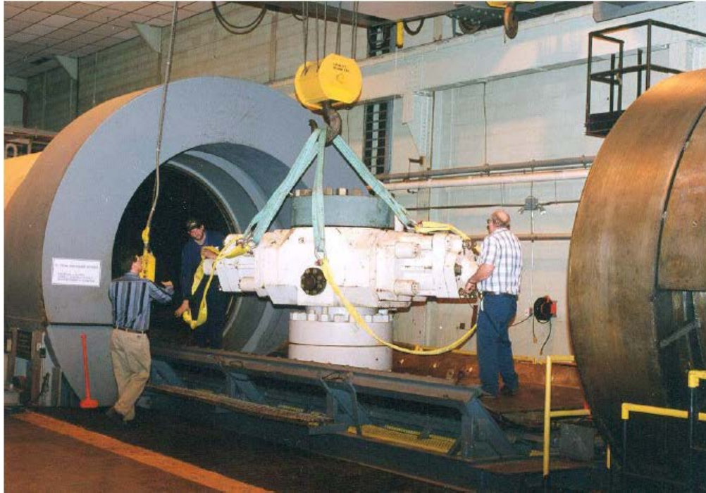
Figure 3.2: Pressure Test of Subsea BOP Section at DOTF Facility [7]
