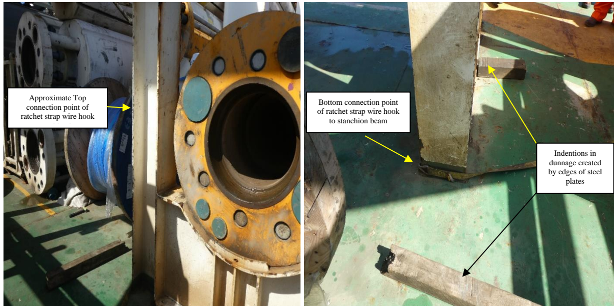
Figure 7 – Dunnage used to support plates on edge and approximate top and bottom connection points of ratchet strap wire hooks.
