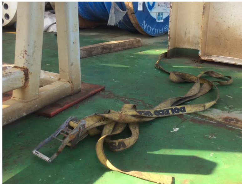
Figure 6 - Ratchet Strap that held the steel plates up against the stanchion beams
