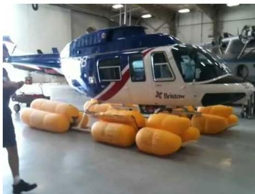
Figure 8. Test of float system deployment
