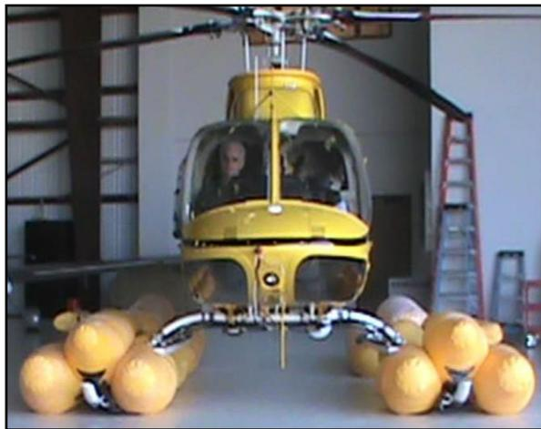
Figure 3. Normal float configuration      Figure 4. Floats activated on Bell 407.
