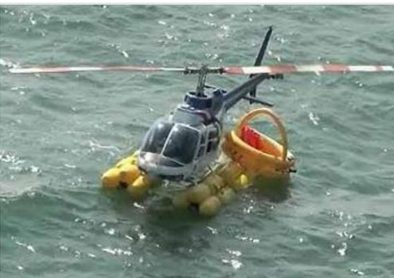
Figure 7. Floats and raft deployed
