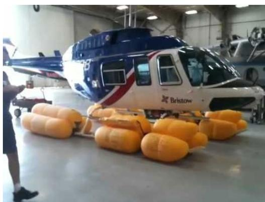
Figure 7. Floats and raft deployed
