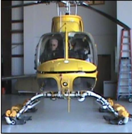
Figure 3. Normal float configuration
