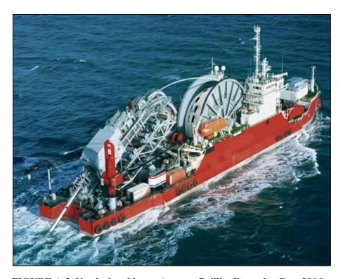
FIGURE A-3 Vertical reel barge (source: DrillingFormulas.Com 2016)
