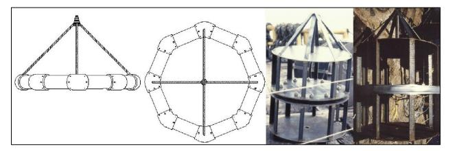
FIGURE A-5 Ring (left) and focusing-configured bulk charge (right) (sources: DEMEX 2003; BOEM staff photo).
