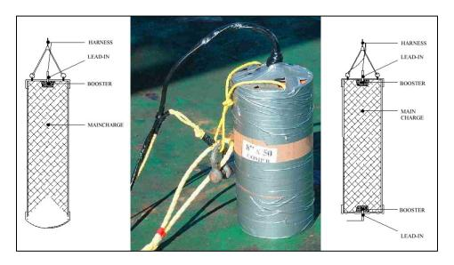
FIGURE A-4 Simple bulk charge design, rigged 50-lb. charge (center), and double-detonation bulk charge design (image courtesy of DEMEX, Int.)
