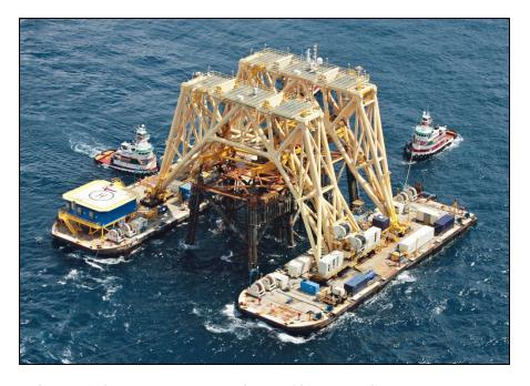
FIGURE A-2 Versabar bottom feeder lift system (Source: Versabar, Inc. 2017)
