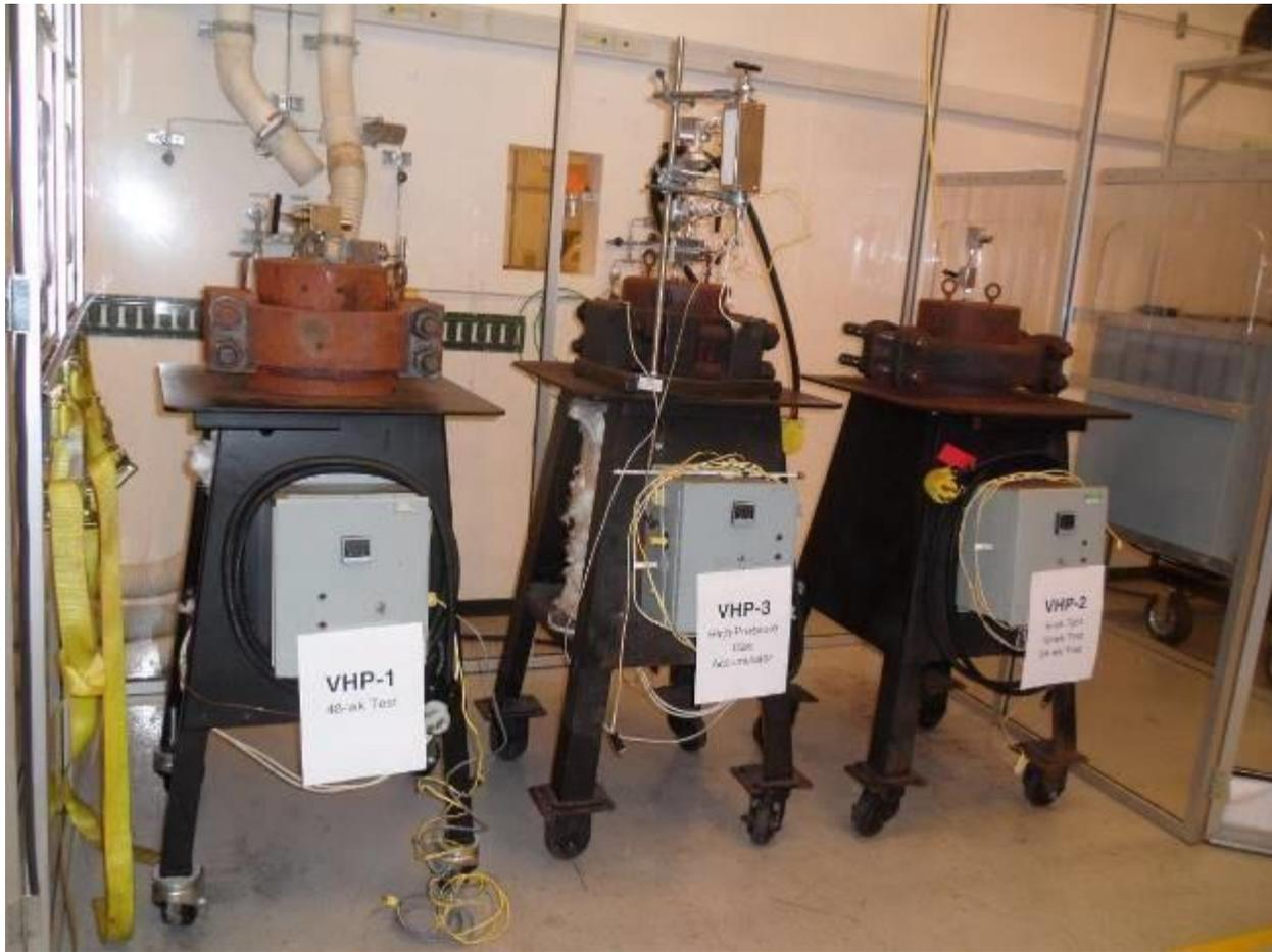
**Figure 1. The three Very High Pressure (VHP) Autoclaves Used for Experimental Evaluation of Cracking Susceptibility**
