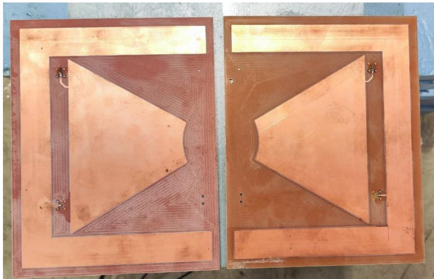
Figure 101: Moving planes sensor with trapezoidal electrodes (with guards)
