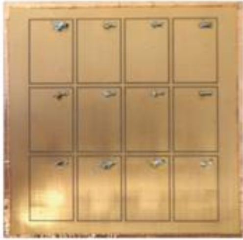
Figure 7: Planar ECT sensor [12]
