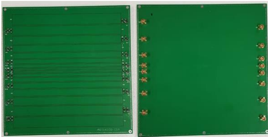
Figure 61: Finalized front view (left) and bottom view (right) of the 16 electrodes sensor board
