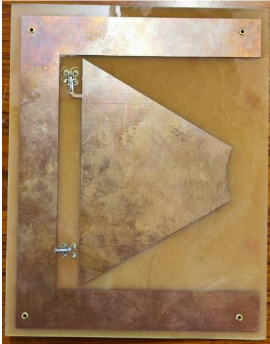
Figure 96: Driven backplane connection to driven guards
