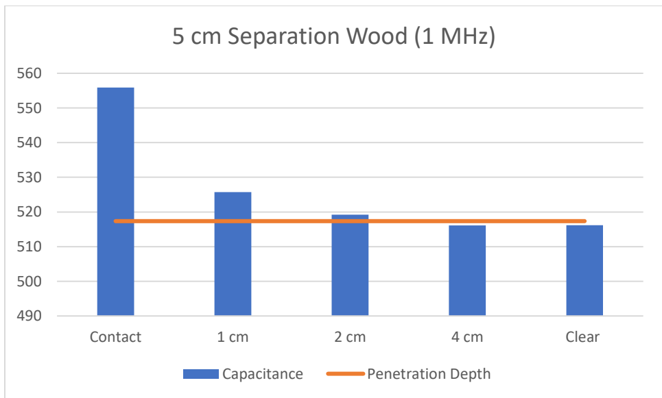
Figure 174: Penetration depth test for 5 cm ice block with the following parameters: 19.5 cm center-to-center separation between electrodes, a wood block as target, and 1 MHz signal excitation
