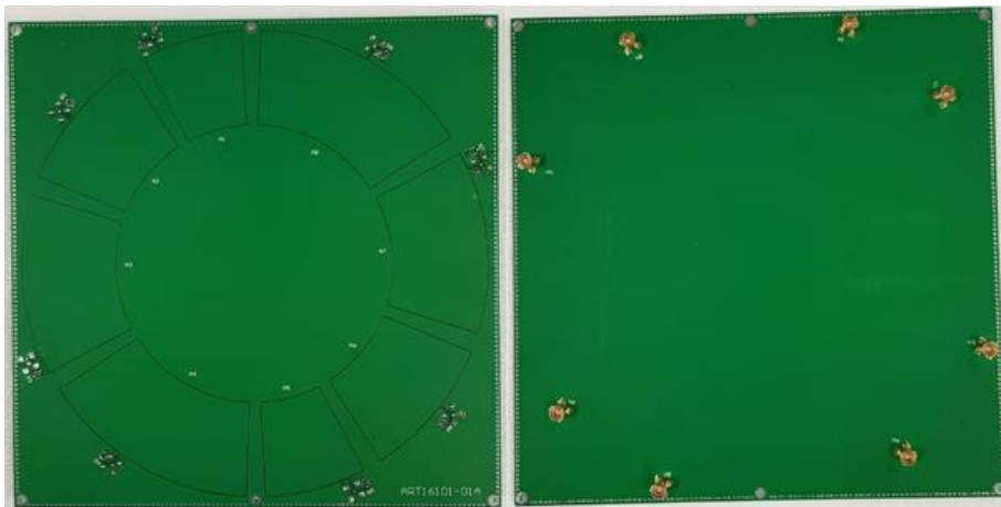
Figure 62: Finalized front view (left) and bottom view (right) of the wheel shaped sensor board
