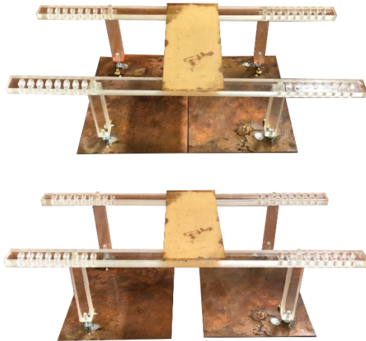
Figure 64: Guide attachment to sensor and movement principle
