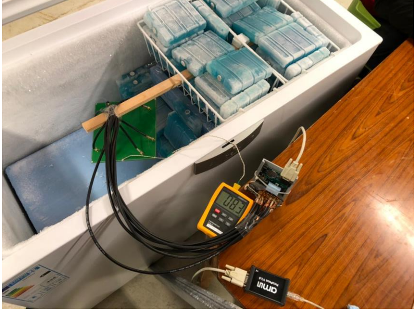
Figure 89: Experimental setup with thermocouple attached to the sensor
