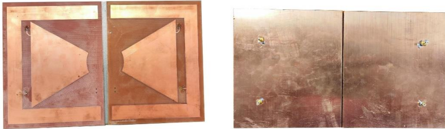
Figure 63: Finalized front view (left) and bottom view (right) of the moving planes sensor with trapezoidal electrodes
