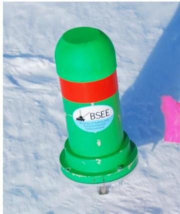
**Figure 18: LDGRIDSAT tag deployed on an ice floe in Alaska**
