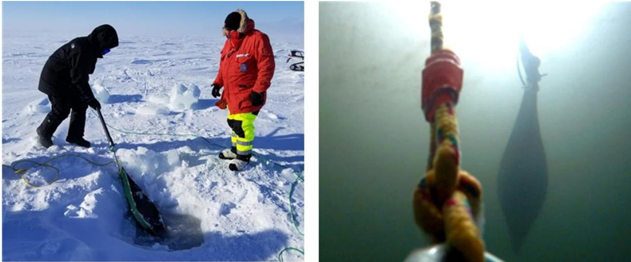
**Figure 24: Deployment of the tethered UWID under the ice floe**
