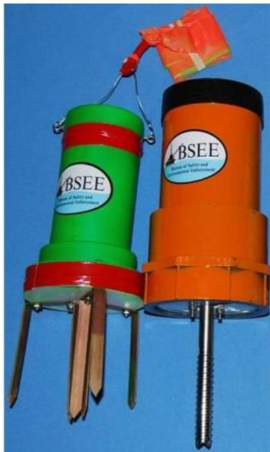
**Figure 4: First generation LDGRIDSAT aerially deployed (left) and surface-deployed (right) prototypes**
