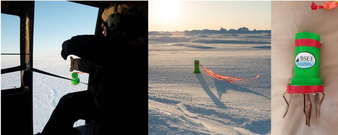
Figure 8: Navy ICEX LDGRIDSAT tag aerial deployment testing
