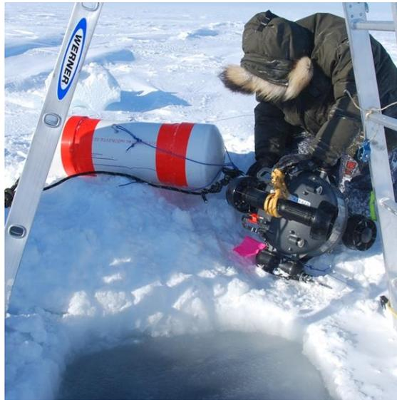
**Figure 26: Deployment of the UWID using an ROV**
