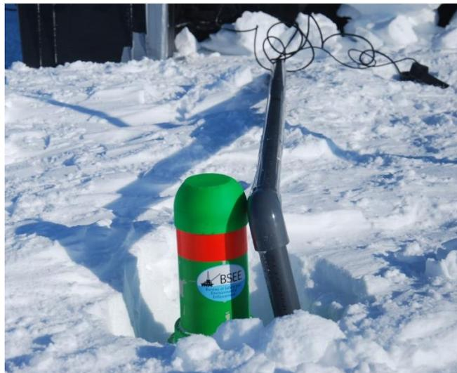
**Figure 25: A tethered accelerometer and LDGRIDSAT tag**
