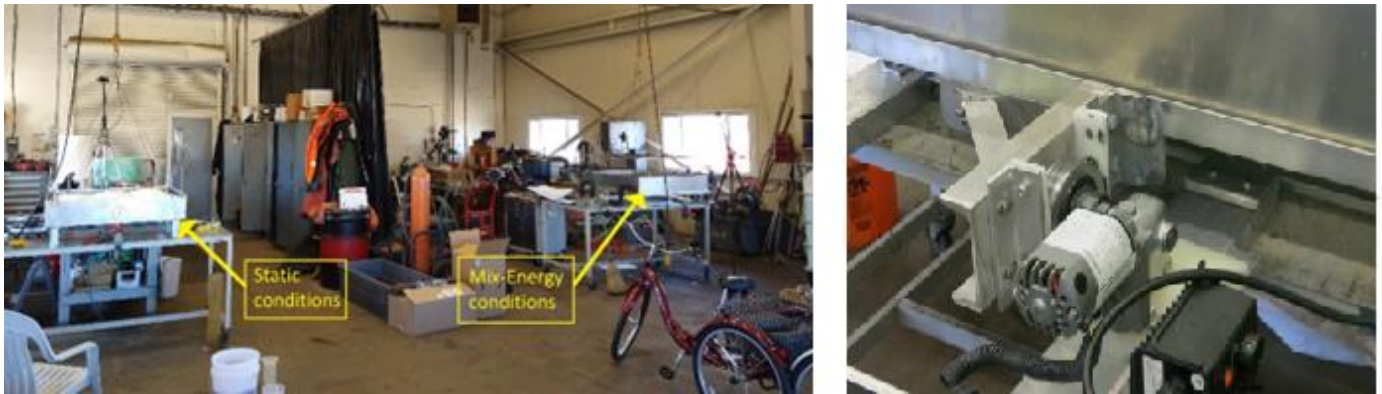
Figure 7. Left: Two test trays for water uptake tests. Right: Eccentric drive used for mix-energy conditions.
