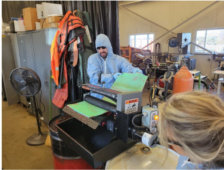
Figure 10. AquaFlex® sorbent sample tested for reusability performance.
