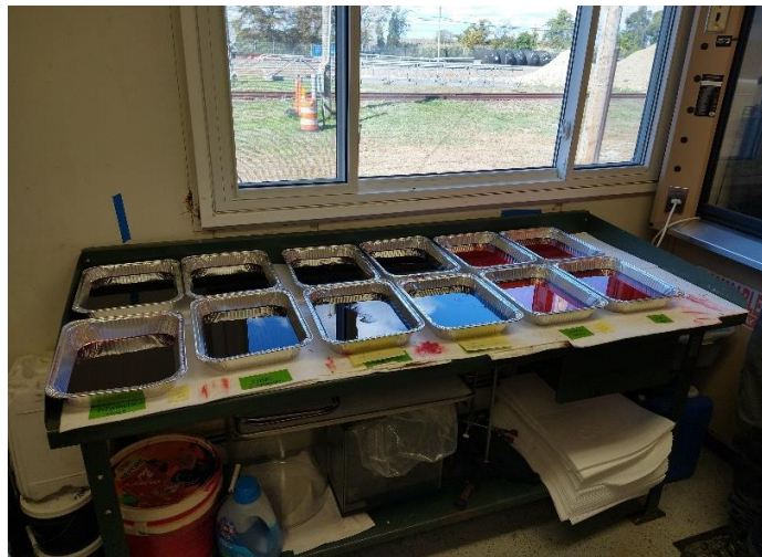
Figure 1. Ohmsett's chemistry lab used for ASTM F726-17 tests.
