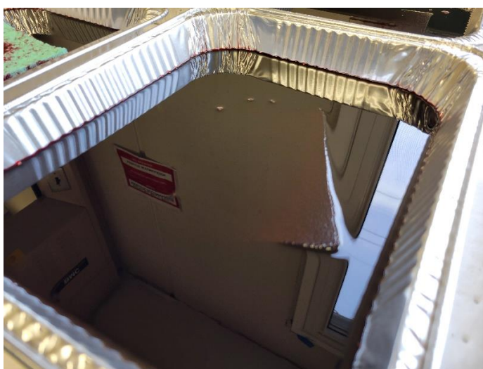
Figure 14. MFNS Technologies' OHM Sponge™ partially sunken in tray filled with Hydrocal 300.
