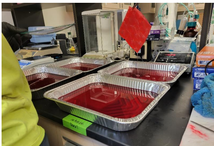
Figure 13. Imbiber Fiber™ prototype sample undergoing 30-second drip time before being weighed in accordance with ASTM F726-17 standard.
