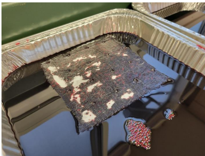
Figure 12. Oil-Only Heavyweight Pad sample floating in tray during ASTM F726-17 tests with Hydrocal 300.
