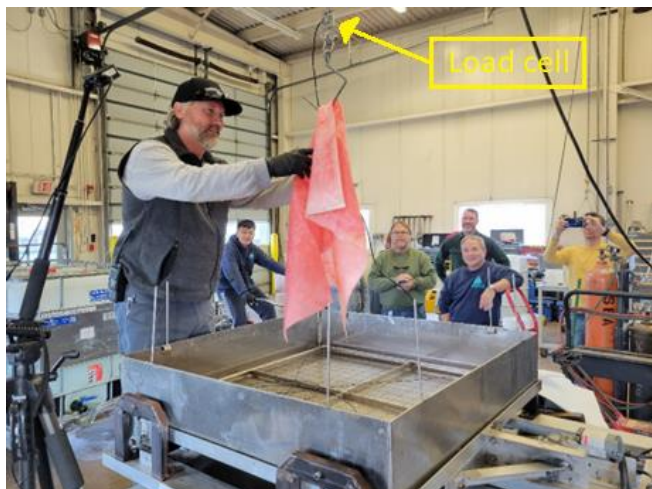
Figure 8. Retrievability test with load cell measuring tear force.
