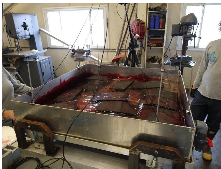
Figure 17. OHM Sponge™ in mix-energy conditions during a water uptake test.
