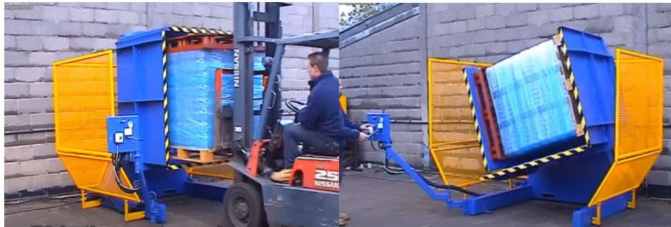
Fig. 10 Pallet inverter used to rotate a stack of ice bins
