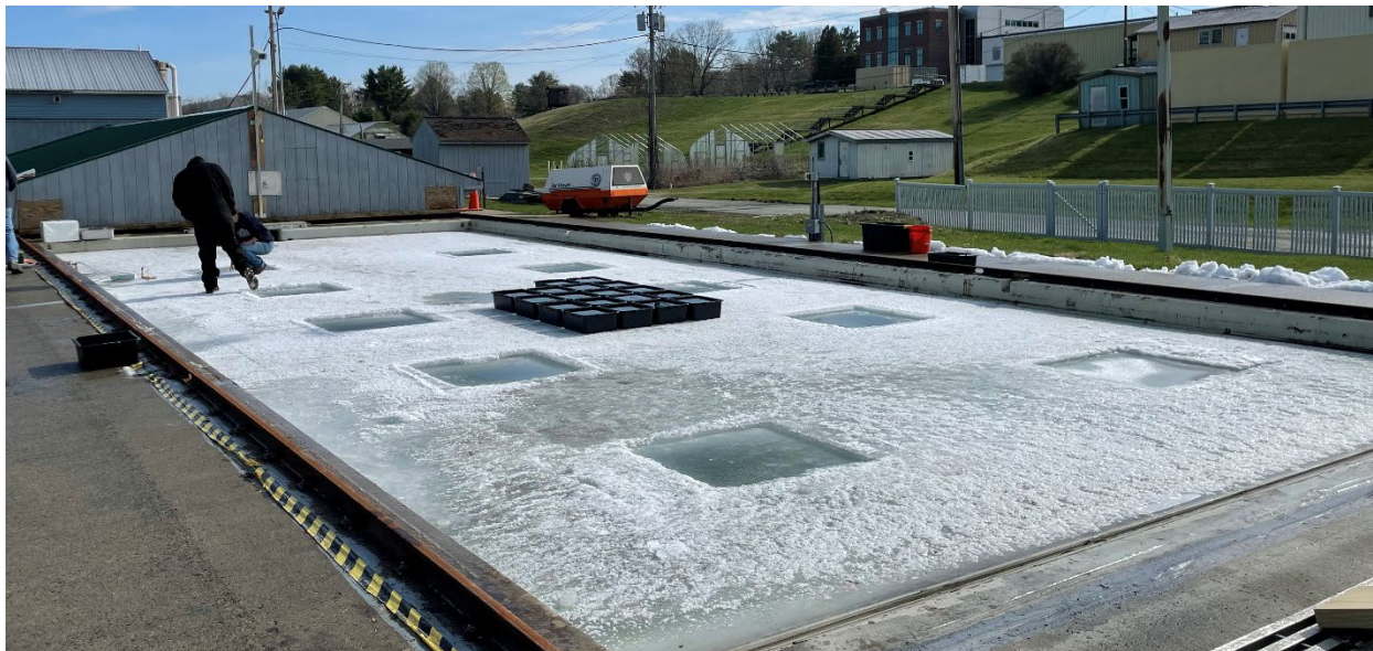
Figure 14. Ground view of the GRF tank with ice squares (1m x1m) and black plastic totes for oil thickness calibration.
