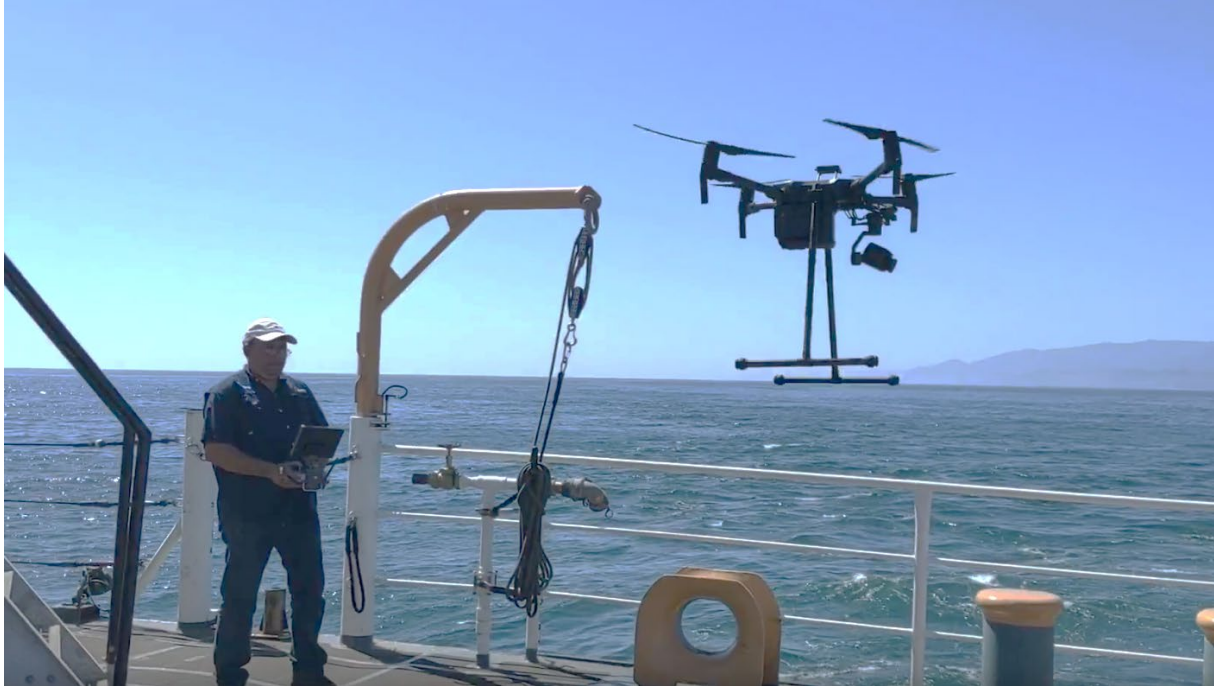
Figure 1 - Previous UAS surveys collected over Santa Barbara seep sites are used on the development of this software. In this image we show a UAS take off from a USCG vessel. The aircraft has a flight time duration of up to 35 minutes and its rigged with a high resolution dual Thermal and Visual camera.
