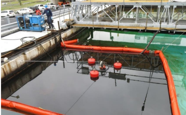
Fig. 2 20 x 20 foot Test Area Used for Weir Skimmer Tests
