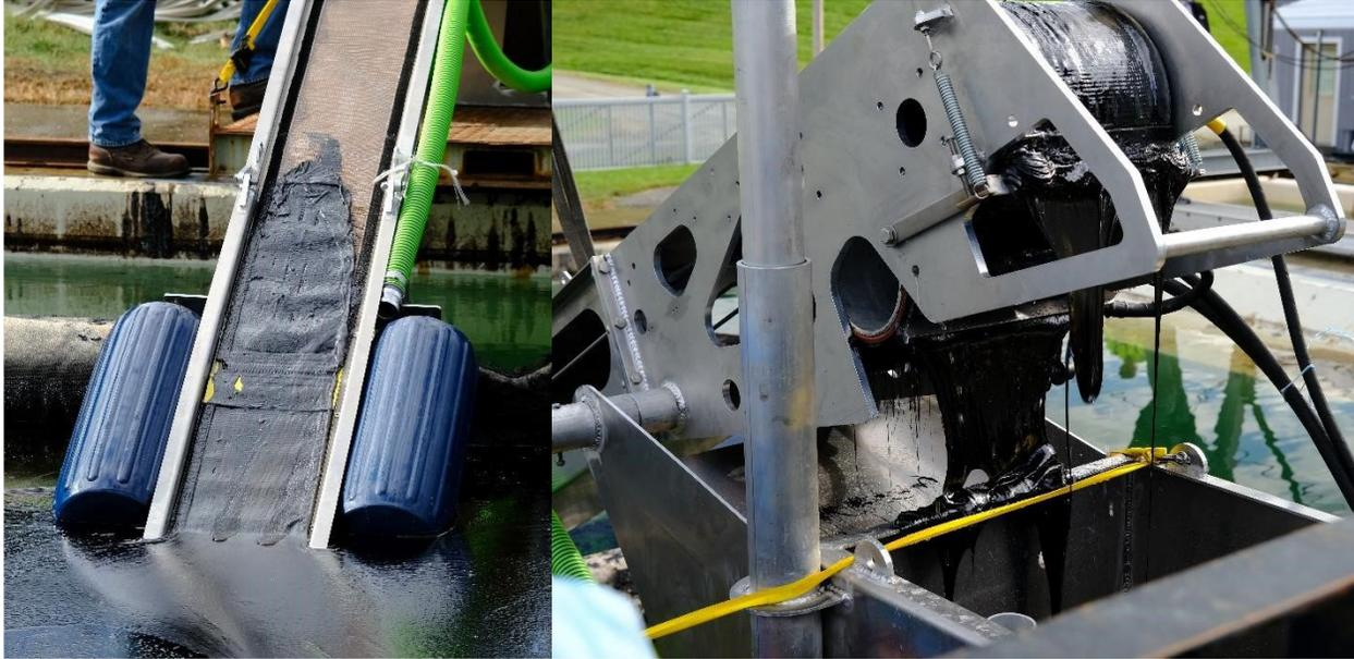
*Figure 13: Elastec Belt Skimmer with Oil*
