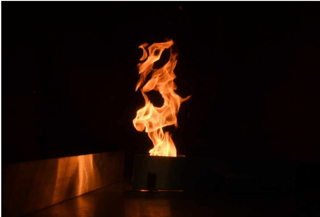
Fig. 9 Photo of flame touching the walls
