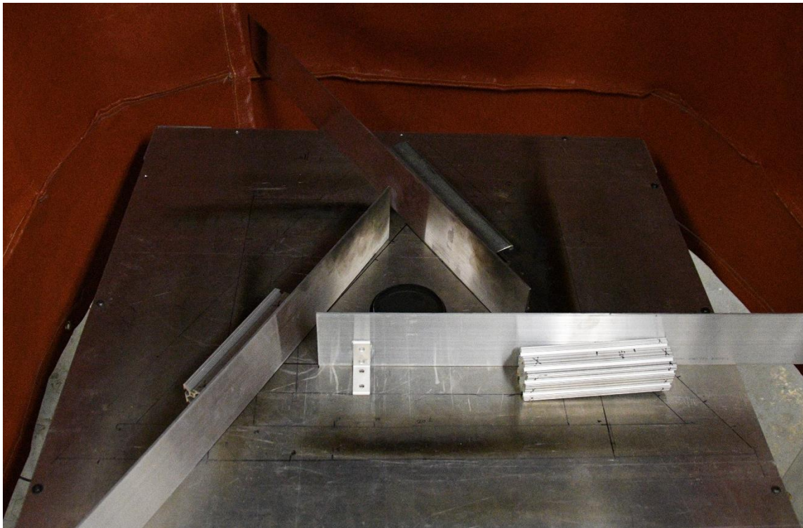
Fig. 8 Photo of three-wall enclosure
