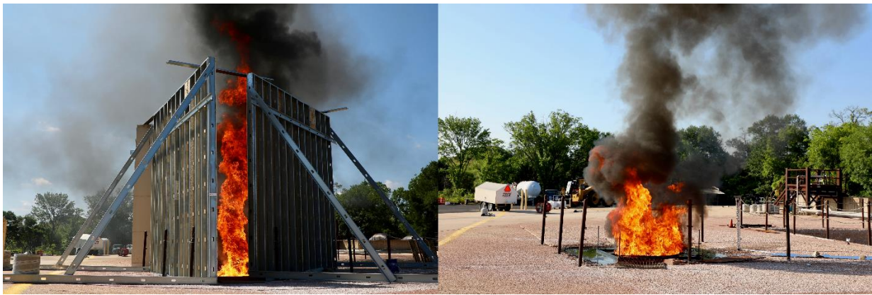
Fig. 37 Fire whirl vs pool fire
