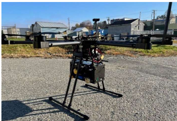
Figure 2-4. U.S. EPA's Kolibri emission instrument system mounted on the undercarriage of the UAS Aurelia X8.
