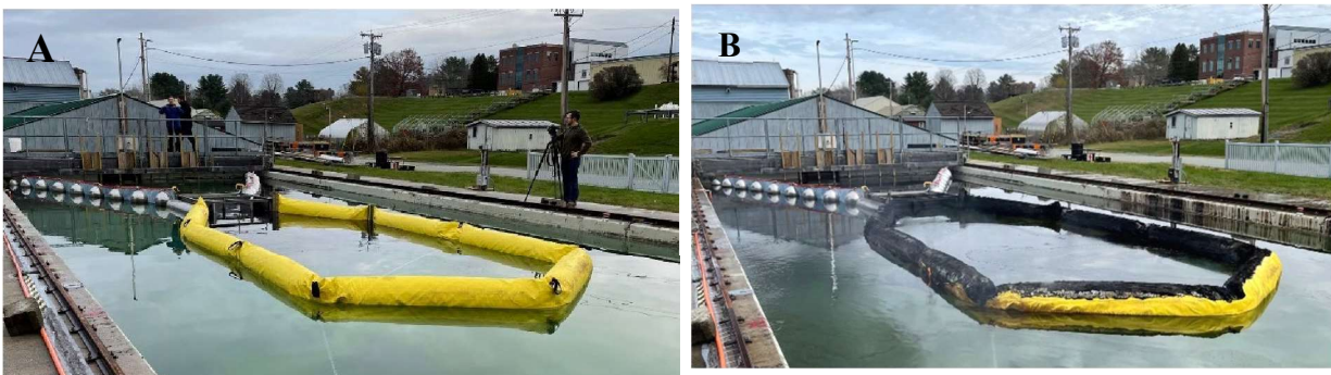
Figure 2-3. Boom configuration A) before and B) after test burn 1.
