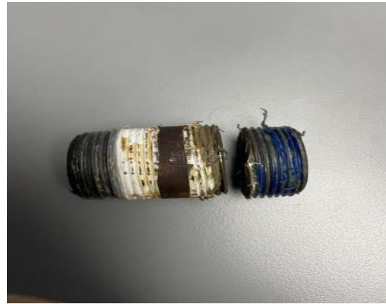
Figure 1-Photo shows damaged 3/4-inch pipe after incident.
