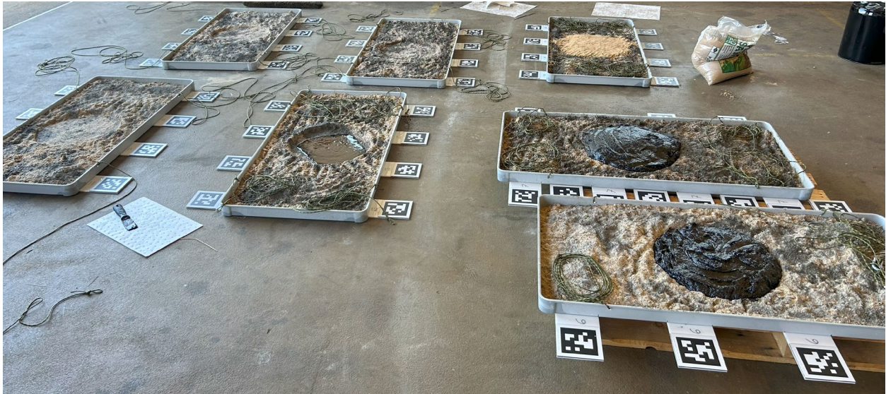
Figure 24: Pans with visual markers and test oils
