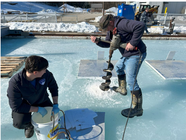
Figure 4: Drilling hole through ice sheet
