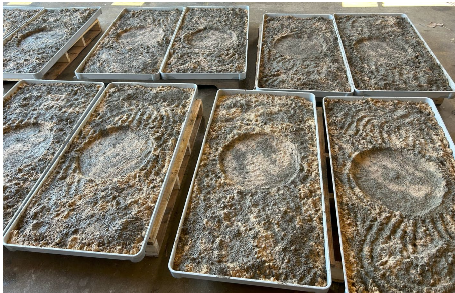
Figure 23: Pans filled with sand and cement mixture
