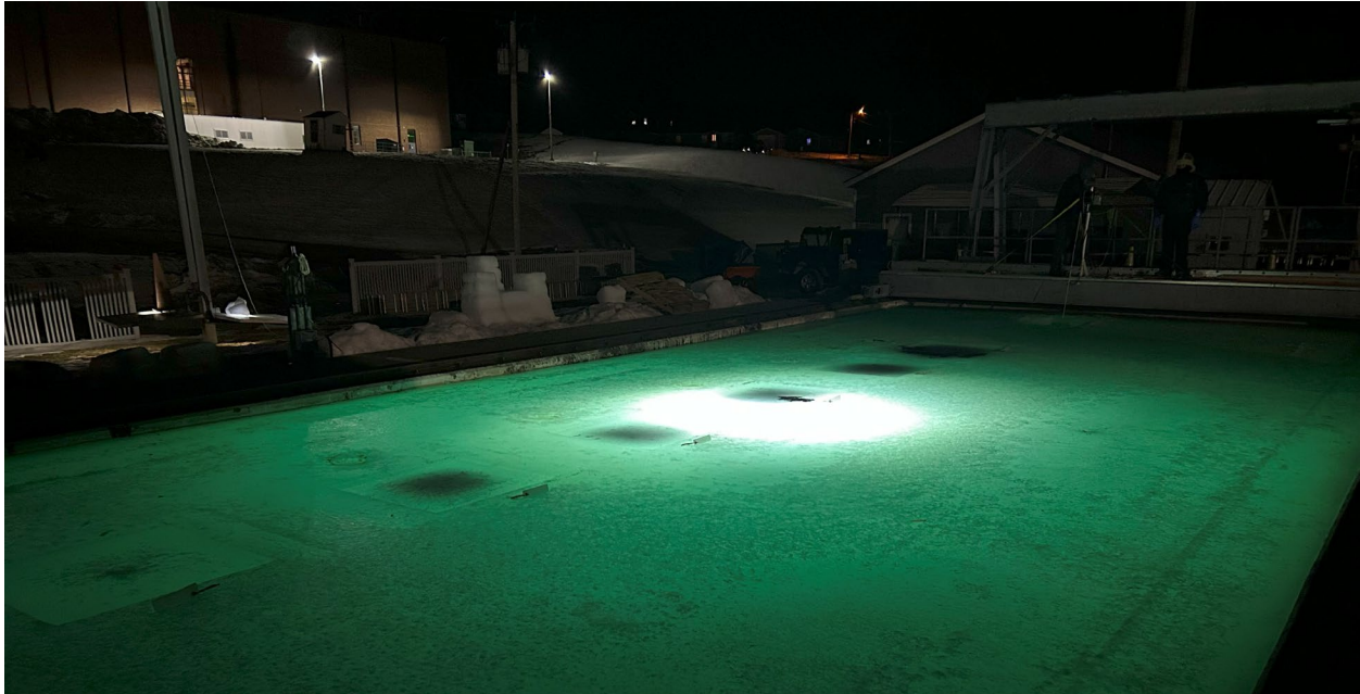
Figure 18: Test areas illuminated from beneath the ice with Sealite LED floodlights
