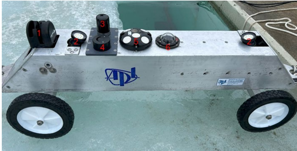
Figure 6: Wheeled cart with sensor payload
