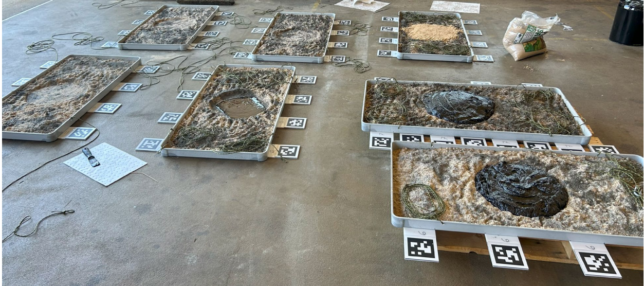
Figure 24: Pans with visual markers and test oils
