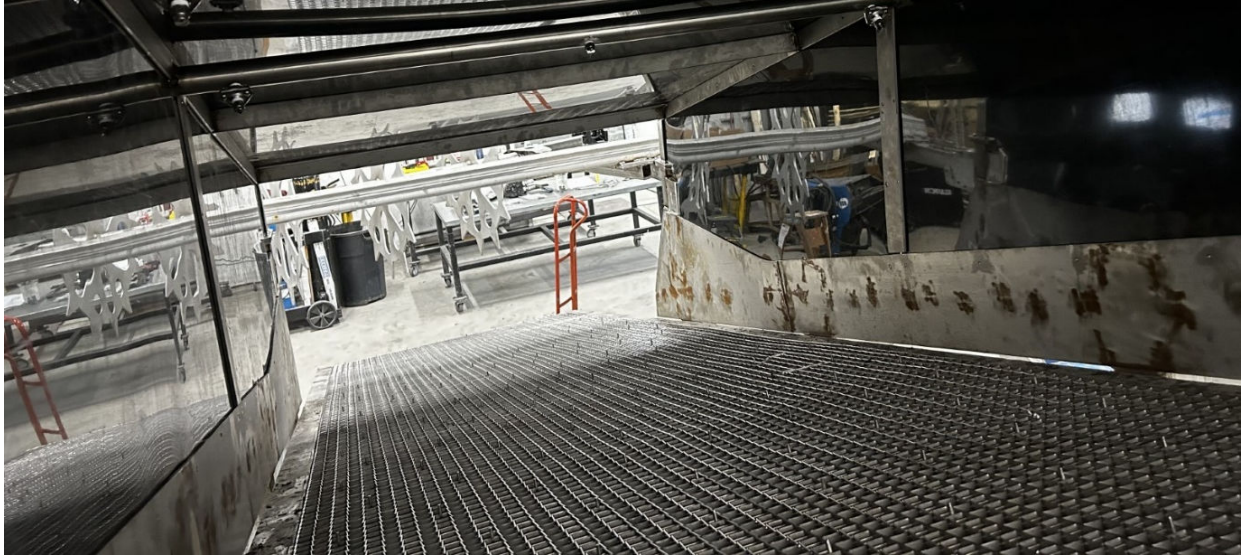
Fig. 7 Photo of inside the spray canopy showing the belt with pin up flights.
