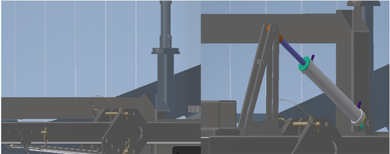
Fig. 4 Proposed hydraulic actuator system on right, original configuration on left.
