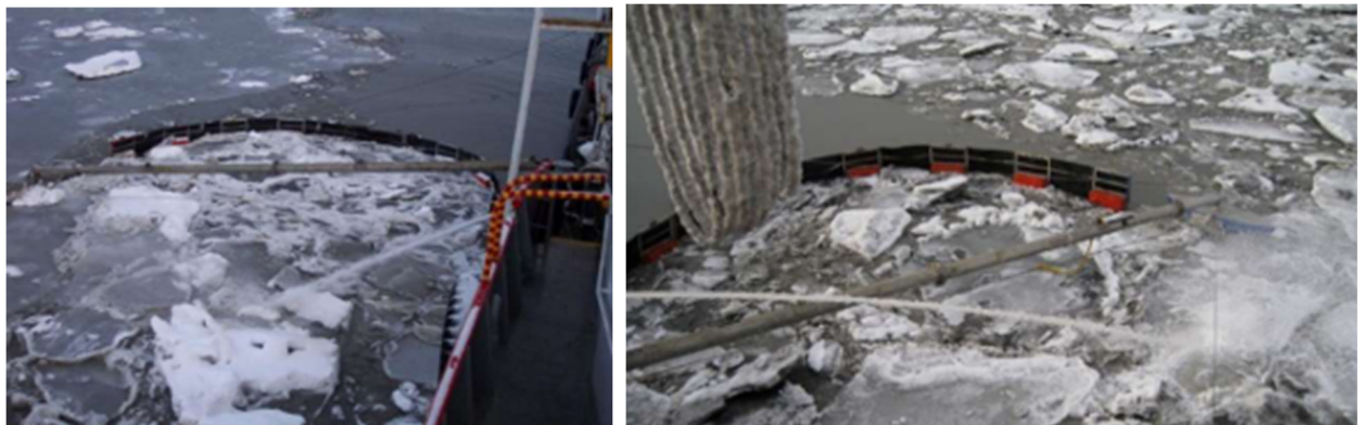
Fig. 34 Ice collected in a containment boom (left) and rope mop skimmer poised above ice ready to recover oil within the ice (right).
