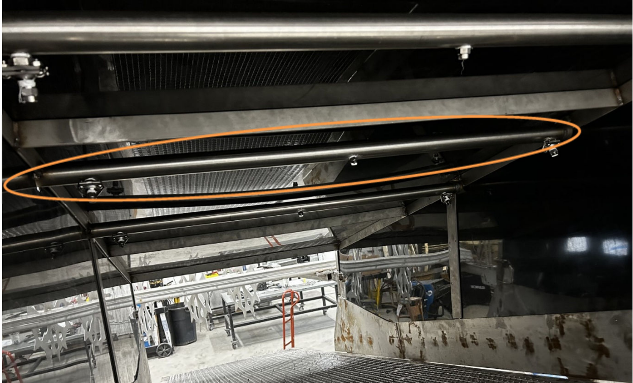
Fig. 24 Photo of inside the spray canopy showing the mounted spray bars (one circled in orange).
