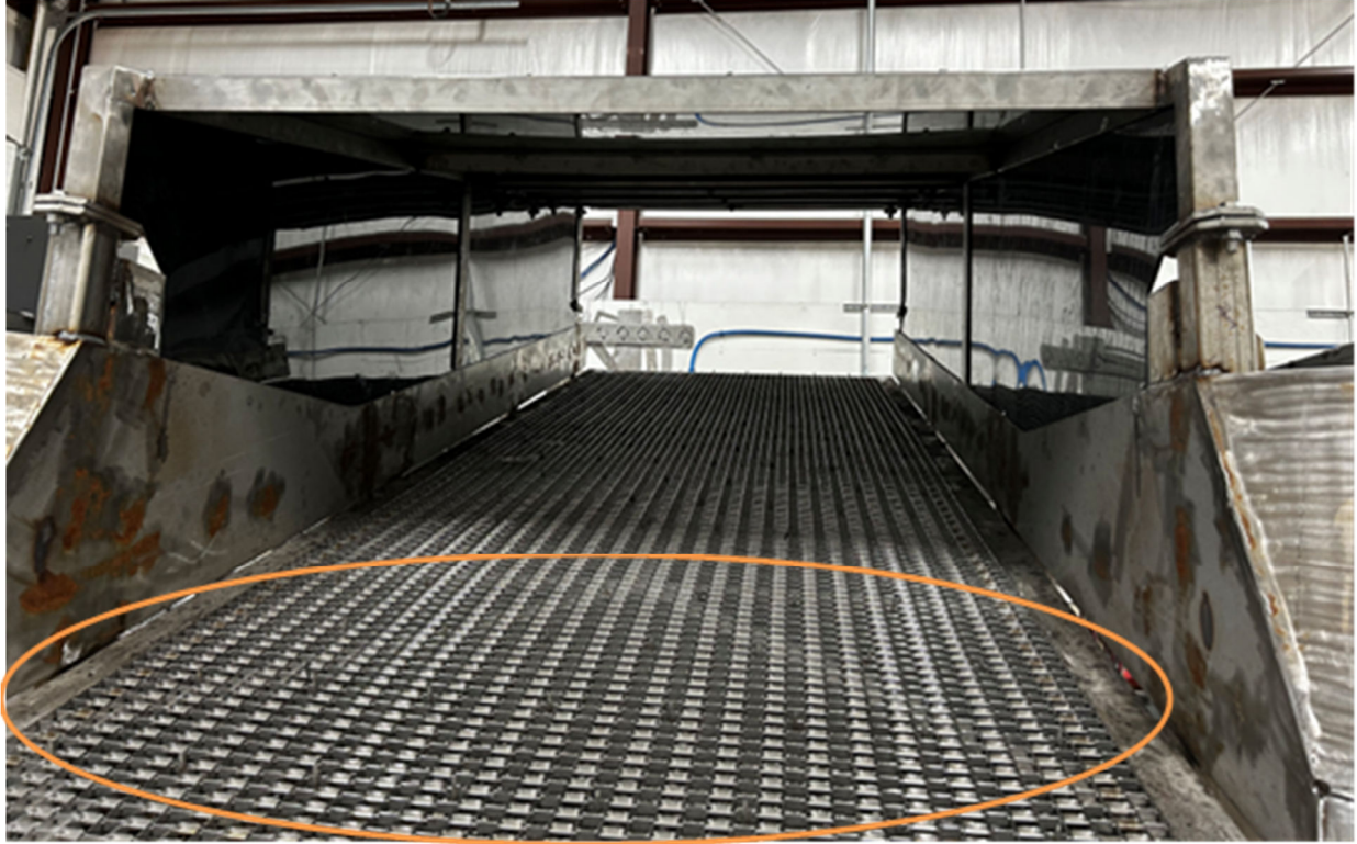
Fig. 17 Photo of reworked conveyor belt – changes to bed circled in orange.
