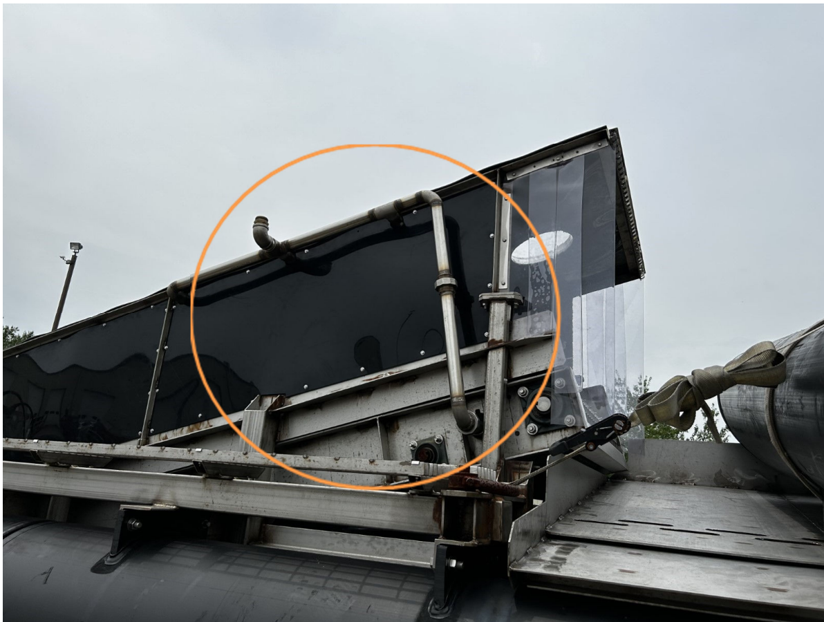
Fig. 23 Spray bar manifold on port side of the frame (circled in orange), with single hose connection at the top, middle.
