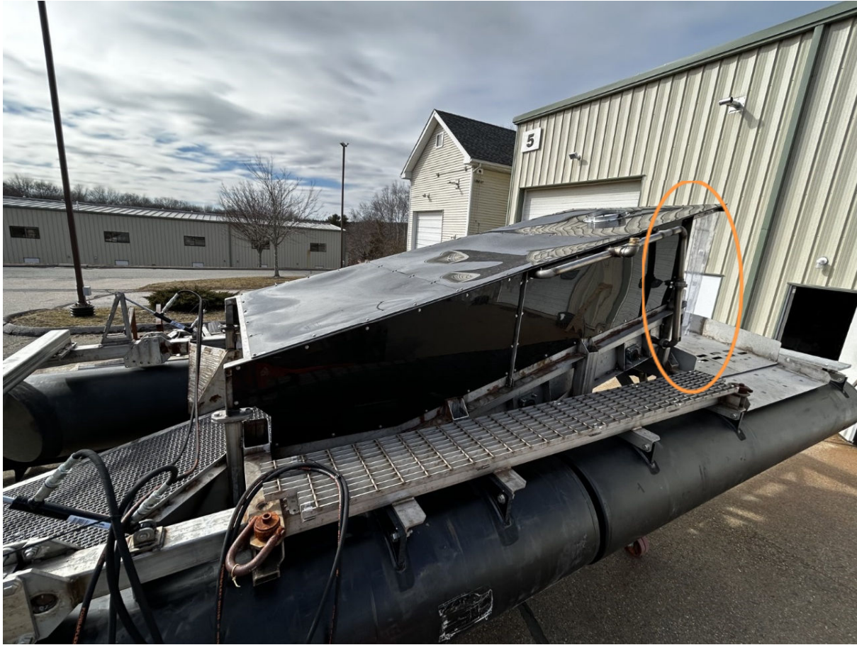
Fig. 25 New solid panel enclosure with flexible strips across the stern to allow the ice to exit (circled in orange).
