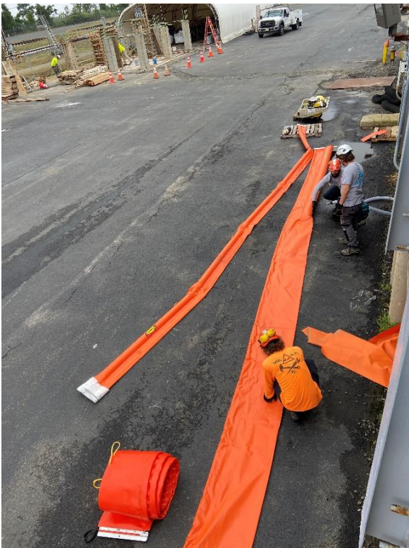
Fig. 4 Abasco quarter and half-size inflatable booms.
