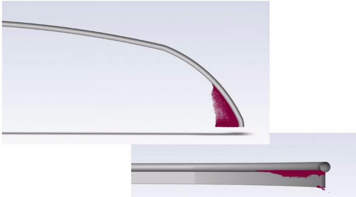
Fig. 55 Abasco, 100%. Cells with oil at 120.92 s and 1.1 kts.
