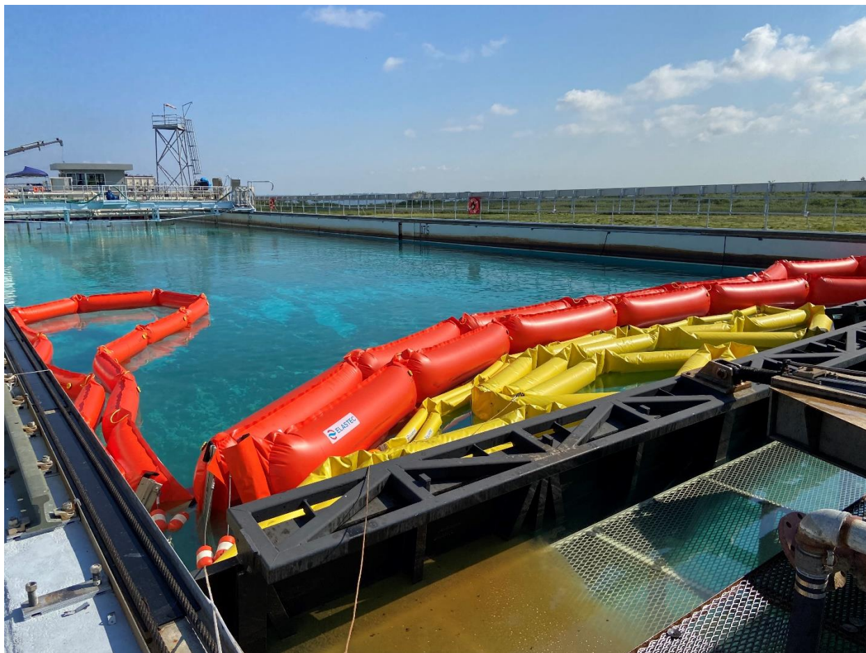
Fig. 5 Booms tied at South end of tank after testing.
