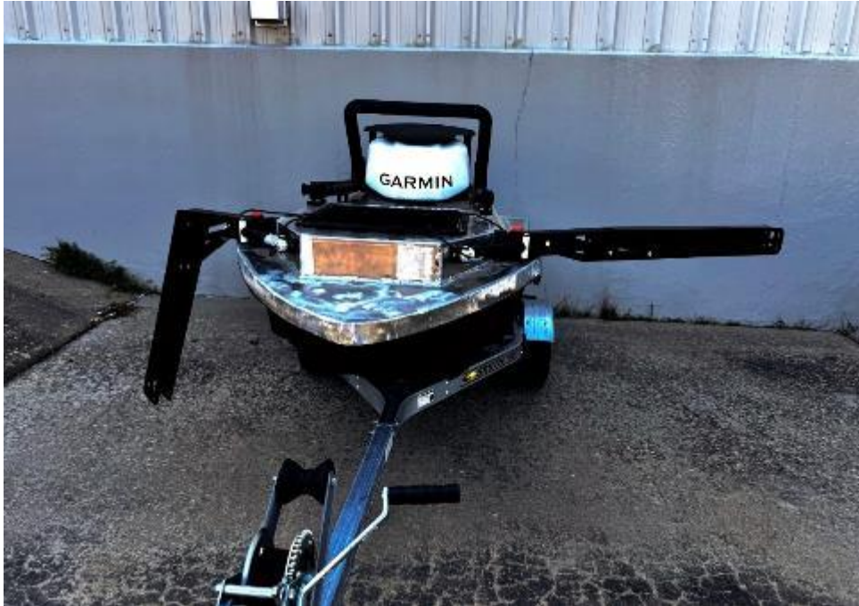
Fig. 11 Hydraulic arms for deploying instruments
