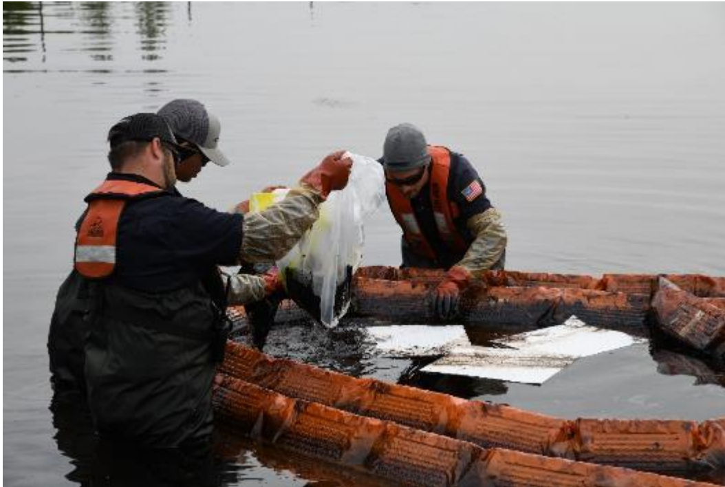
Fig. 15 Cleaning oil from the test basin
