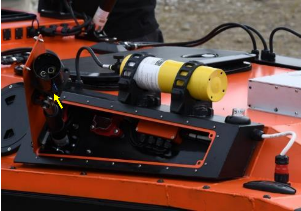
Fig. 8 Herder and ignitor port
