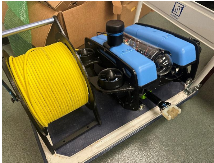
Fig. 16. New BlueROV2 Heavy integrated with scanning sonar and gripper.
