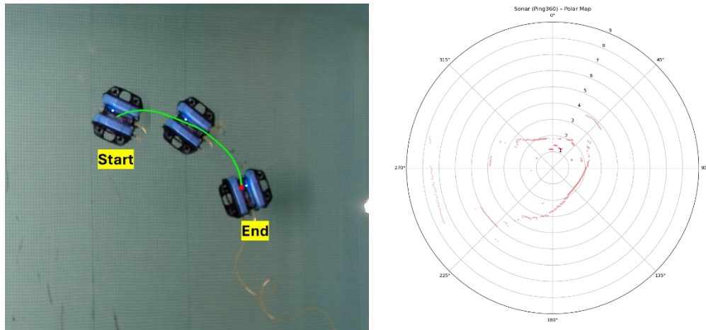
Fig. 26. Left: Top-down view of ROV motion without active stabilization. Right: Corresponding sonar mapping during free roaming for a swimming pool.
