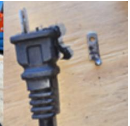
Figure 3-Melted Plug to Tubing Bender
