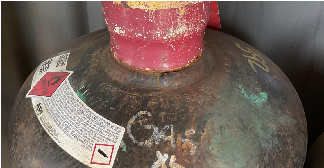
Markings and Labels on Compressed Gas Cylinder on Drilling Rig During BSEE RBI
