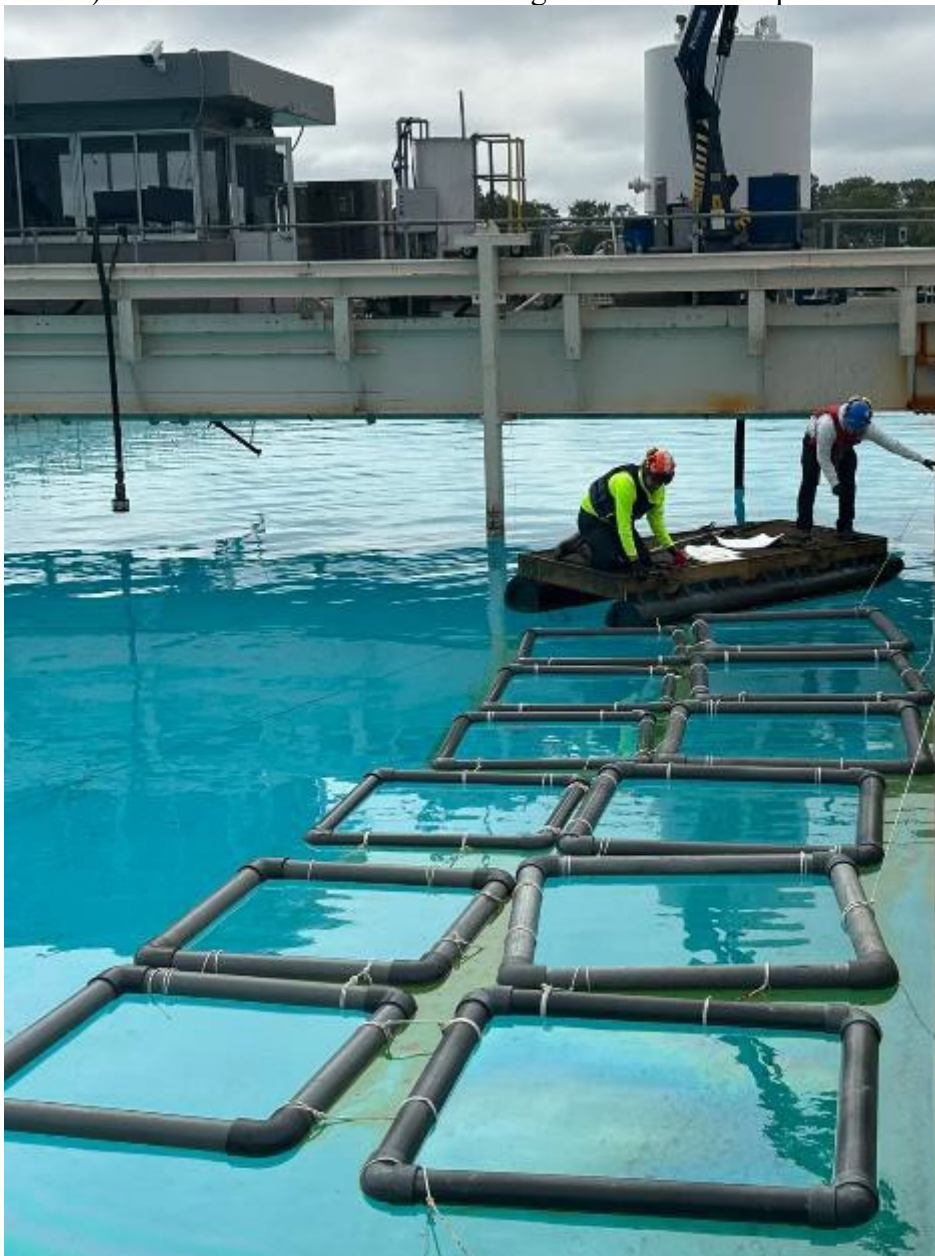
Figure 16. Floating targets inside the Ohmsett tank.
