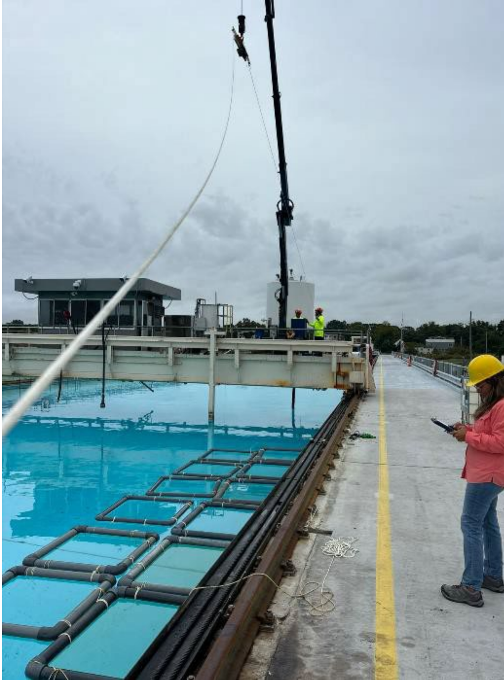
Figure 17. Collection of imagery over the squares using the sensors mounted on the crane. In this case there were overcast (cloudy) conditions. All the environmental variables were recorded associated with the remote sensing data.
