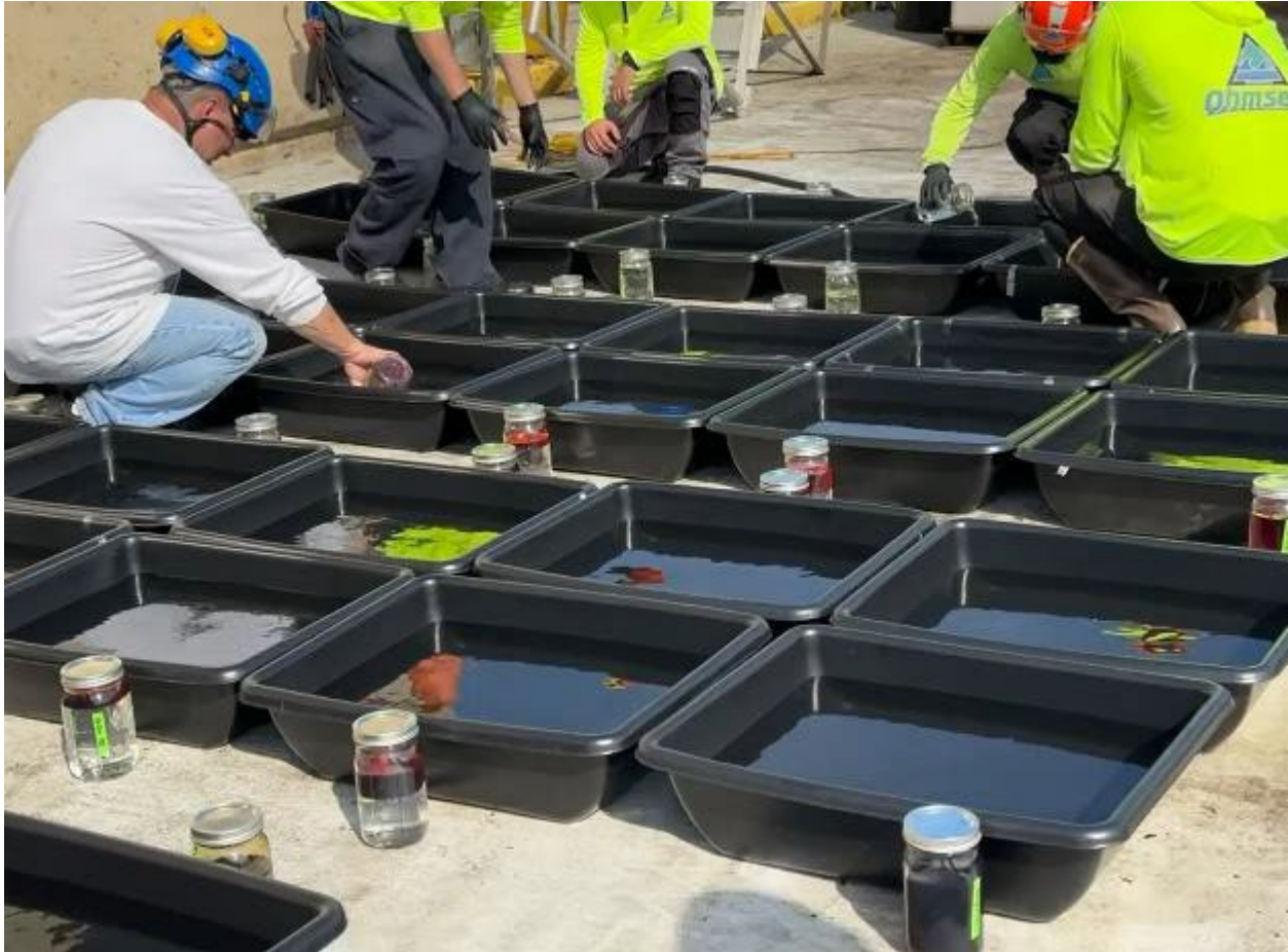
Figure 12. Setting up the DF thickness targets outside the tank. In total 46 plastic containers were used. All the plastic containers were filled with the same volume of water, then known amounts of DF were added to generate a variety of DF thickness layers.
