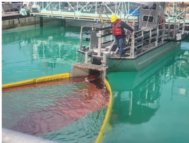
Figure 12. Kvichak vessel with X30 grooved disc skimmer collecting dielectric fluid after waiting for fluid to pool in the intake area.
