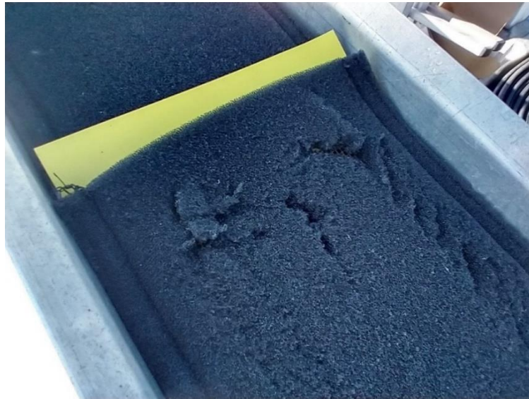
Figure 19. Damaged sheen pads on the Marco FilterBelt skimmer due to wear and tear.
