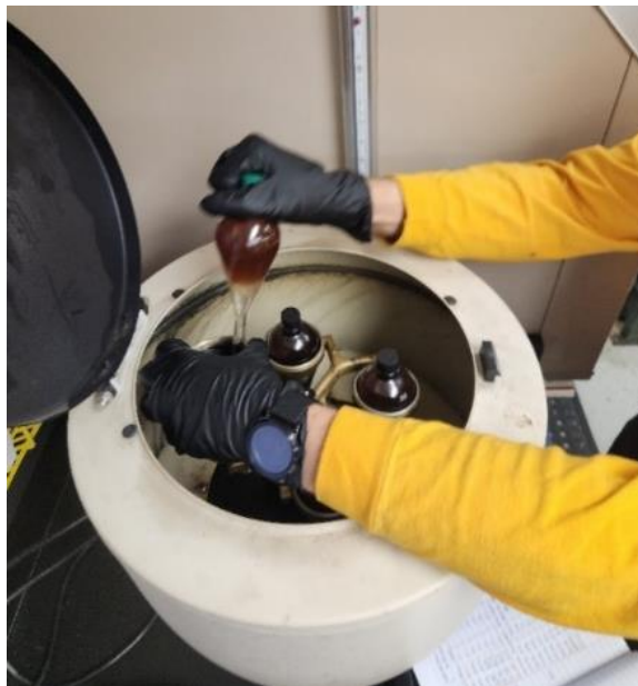
Figure 10. Using a centrifuge in Ohmsett’s chemistry lab to determine a sample’s water content.
