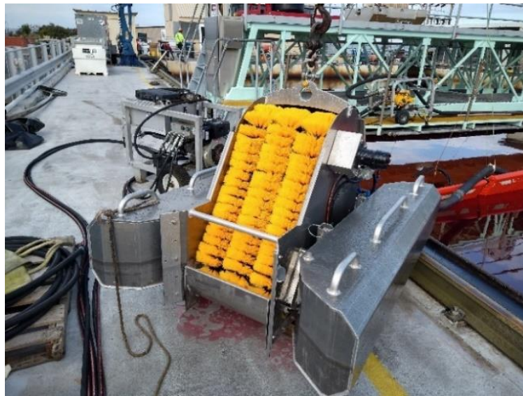
Figure 3. Lamor MultiMax 50 brush skimmer on Ohmsett's deck.
