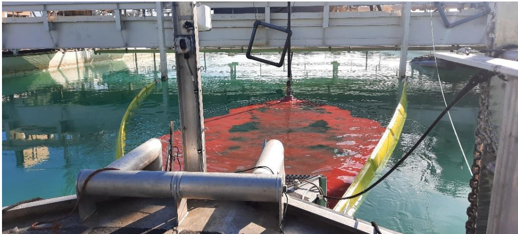
Figure 11. Dielectric fluid being released from a discharge pipe on the main bridge and floating towards the Kvichak vessel during an advancing skimmer system test.
