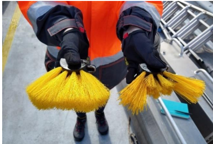
Figure 4. Two different Lamor brushes used for experiments. Left: Alternate (long/dense) brush. Right: Standard short brush typically used in most Lamor brush-skimming operations.
