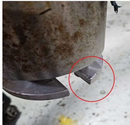
Figure 2: (Incident 1) Scarring observed on the anti-two block.
