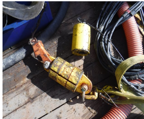
Figure 2-A2B cable failure resulted in the weight falling directly onto the deck.
