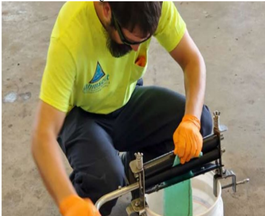
Figure 6 Application for Field Scale Test Protocol for Type I Sorbents 2021, Manual Roller System
