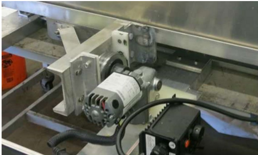
Figure 3 Application for Field Scale Test Protocol for Type I Sorbents 2021, Variable Speed Motor drive unit
