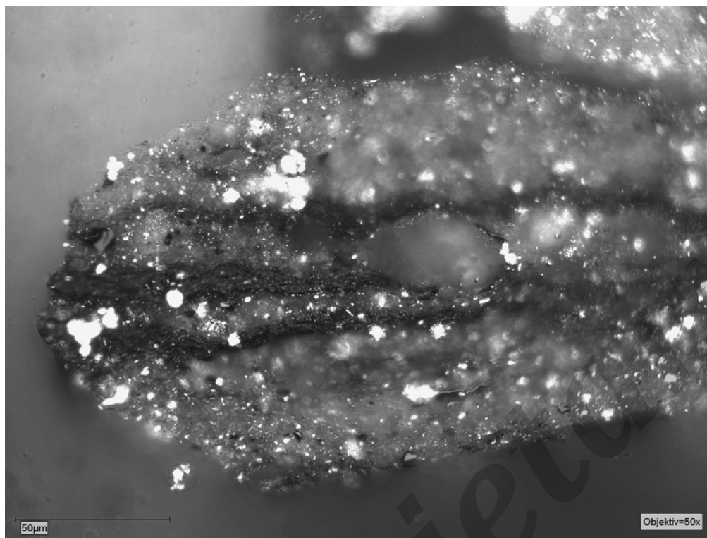
E1934E – GC1191-3 - Lamalginite and bituminite in claystone, reflected white light, X50
