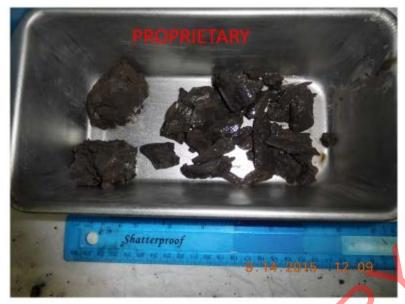
Circulating inside of the casing show with flow rates of 833 gpm versus 445 gpm when pumping out of hole. Hole unloaded well before bottoms up. Material over shakers were approximately 70% Soft Claystone and 30% Hard Shale Cavings.
