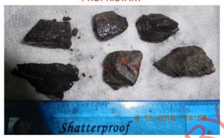
The rig short tripped 5 stands and went back to bottom. The hole was circulated with a slightly increased volume of material over the shakers. The cavings consisted of hard Shale cavings noted in previous slide as well as splintered, brittle Shale.
