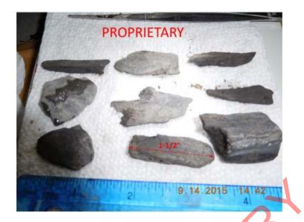
Hydrated Claystone cavings with worn off edges.
