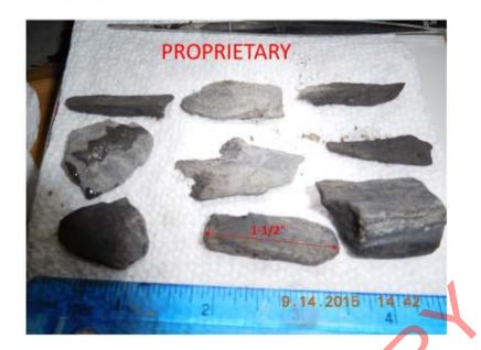
Hydrated Claystone cavings with worn off edges.
