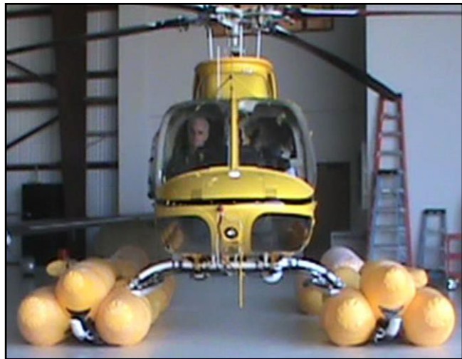
Figure 4. Floats activated on Bell 407. for a Bell 407
