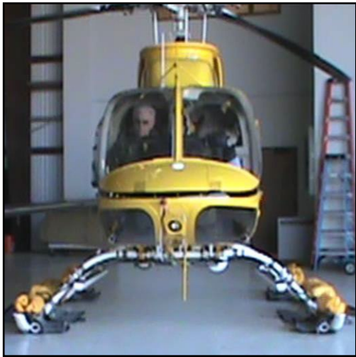
Figure 3. Normal float configuration
