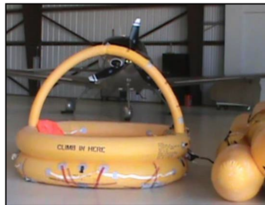
Figure 6. External life raft deployed.
