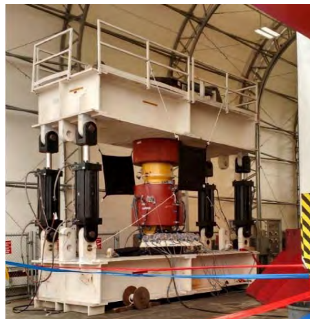
Connector Testing (Combined Loading: Pressure, Tension, and Bending)
