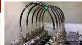
Hose Cycle Testing
