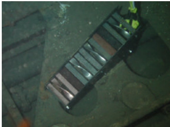
Figure 5. BART Test Platform set at the U-166 site.
