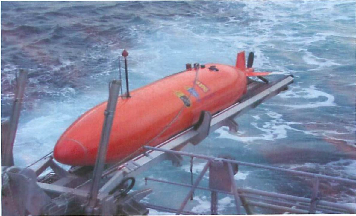
Photo 1 Photograph of the AUV on the vessel in preparation for launch
