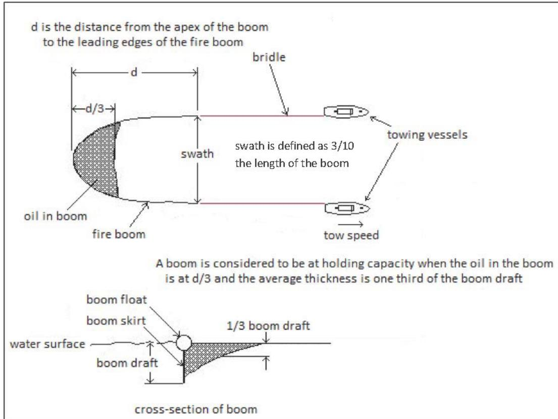
Figure 1. Advancing Burning System Components and Definitions.
