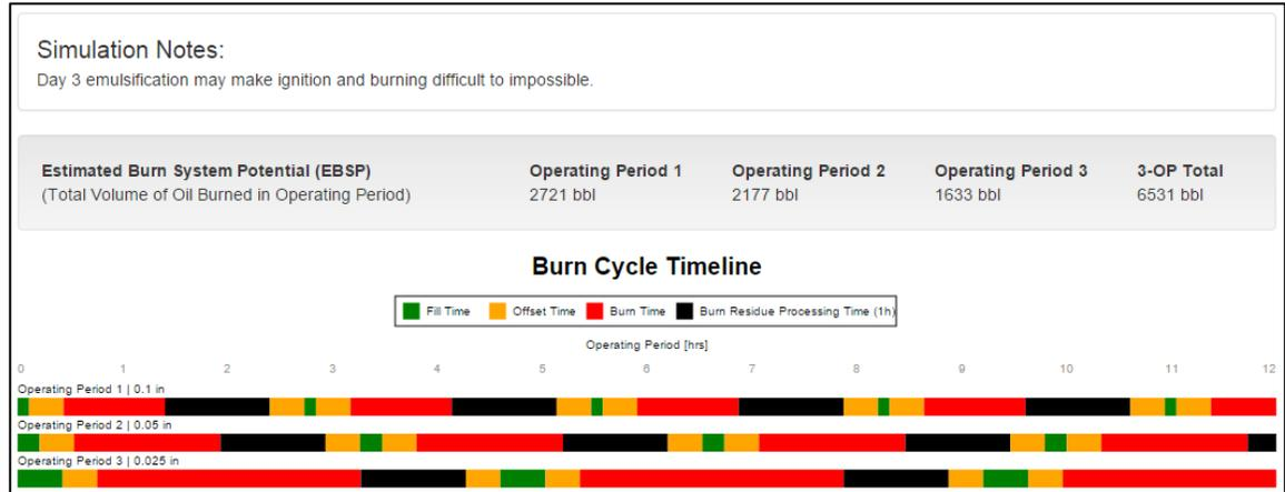
Figure 19. EBSP Graphical Outputs for Burn 1 Batch Spill with Enhanced Collection Configuration.
