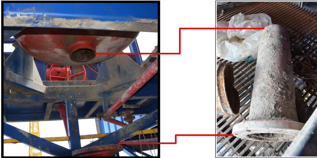
Figure 18: Post-Incident Photographs of the MGS Section of 8” Drain Outlet Piping after Cutting and Removal.
