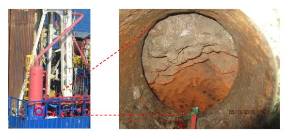
A BSEE Panel investigation identified a number of established Safe Work Practices (SWPs) that, if followed, should have prevented the task from proceeding in the manner in which it occurred. The contaminating material, believed to be cement, had already begun to cure and harden inside the MGS when it was discovered. The decision was made to attempt to remove the material, and supervisors authorized the task without understanding of the extent of the buildup.
